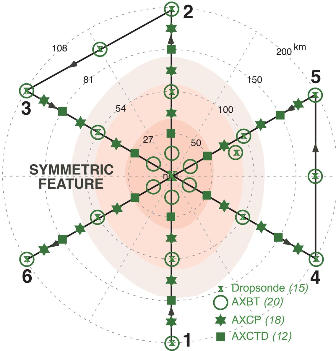
**Fig. 1. (b) Pre-storm Ocean Survey Pattern**
