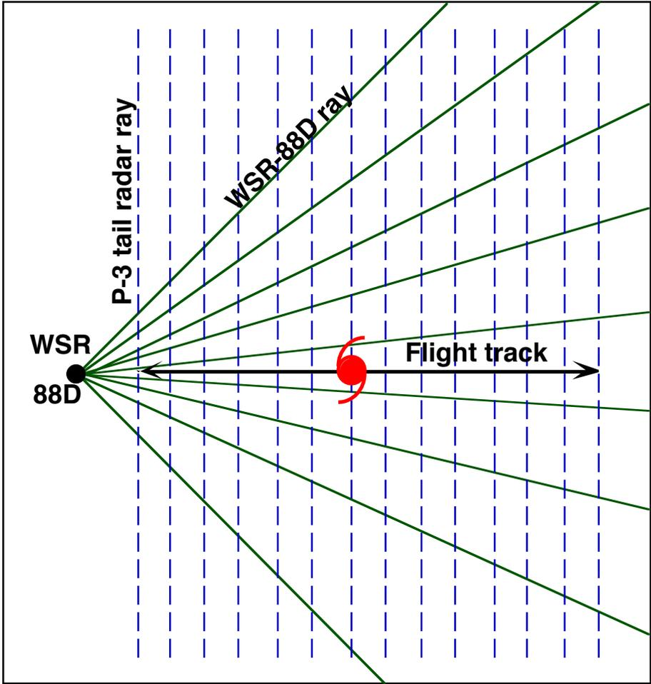
**Fig. 10. Ground-based/Airborne Doppler Scanning Strategy**
