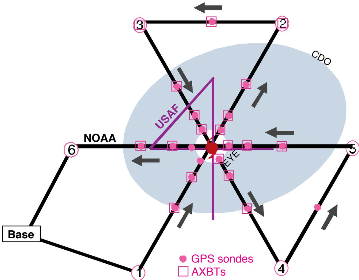
**Fig. 6. Basic (STAR) Flight Pattern**
