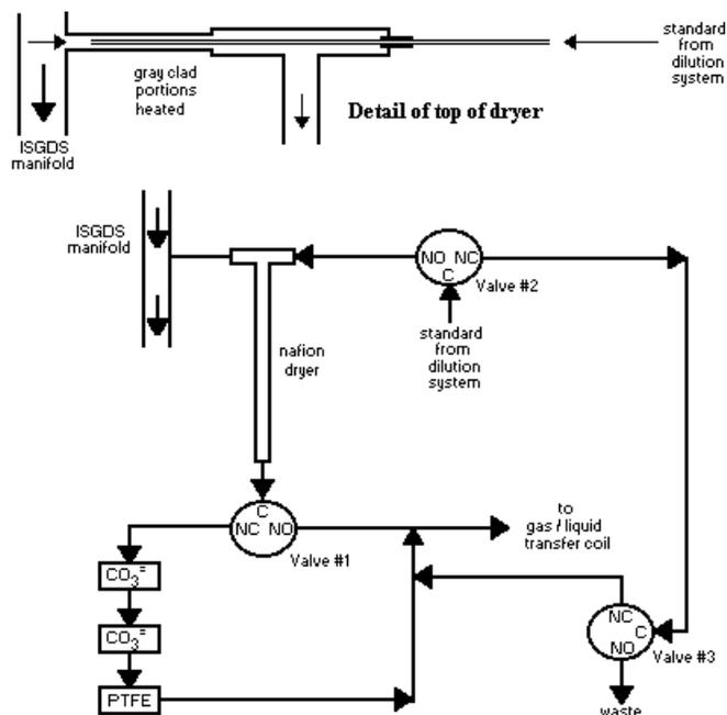
Figure 1. Schematic of the HPLC/fluorescence instrument.
