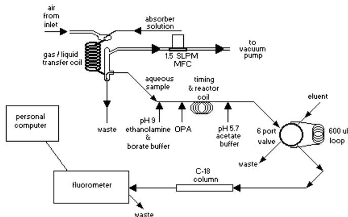
Figure 2. Schematic of the inlet used on the HPLC/fluorescence instrument at GASIE during intercomparison periods 2b-4.
