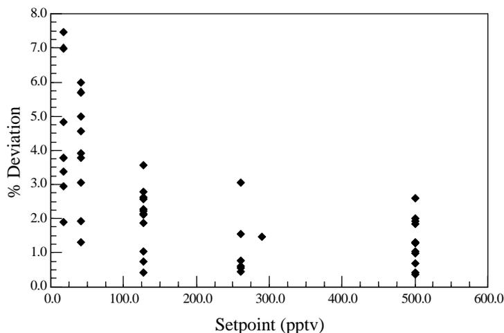
Figure 4 - Precision of the HPLC/Fluorescence instrument during the GASIE intercomparison. The data shown are  $1\sigma$ /SGDS setpoint of the replicates for each measurement period, plotted against the SGDS setpoint.
