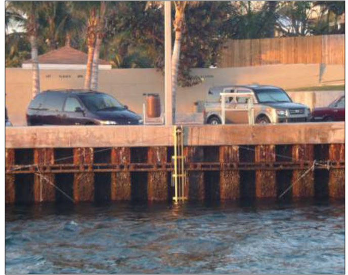
Figure 4. The flow measurement system mounted on the north bulkhead of Boynton Inlet.
