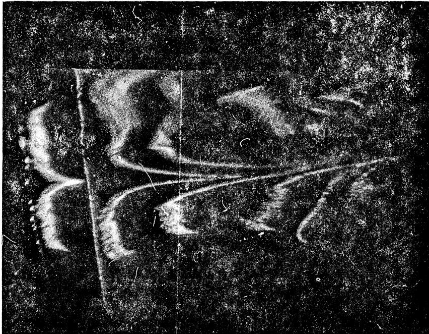
Figure 1. Bubble lines and surface reflections. The width of the photograph represents 24 mm in the direction of the flow. A curved line of bubbles is just leaving the electrolysis wire on the left, and the surface reflection gives a symmetry about a horizontal line. The vertical out-of-focus white line is the wire of a wave gage.
