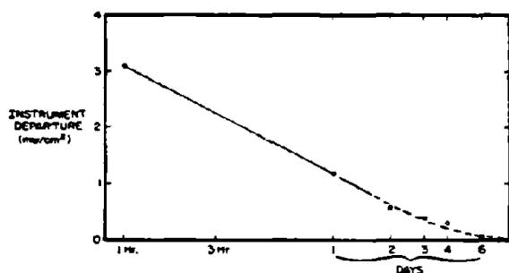
FIG. 7. Departure of pyranometer sensor due to random errors in measurement. Time indicates the period over which the data are integrated.
