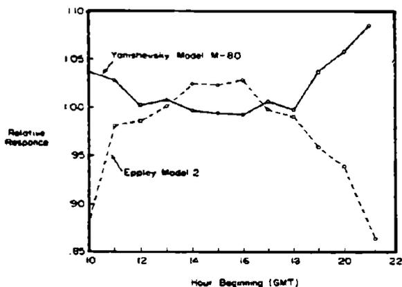
FIG. 5. Relative response of a group of Yanishevsky pyranometers (Nos. 43, 2, and 5373) and a pair of Eppley pyranometers (Nos. 11539 and 12159) during the period 2-9 August 1973, showing the variation in response due to sun elevation angle.
