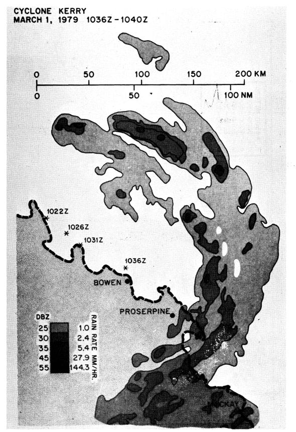
Figure 77. Digitized Plan Position Indicator radar depiction of Tropical Cyclone Kerry compositied from 1036 Z to 1040 Z on March 1, 1979.
