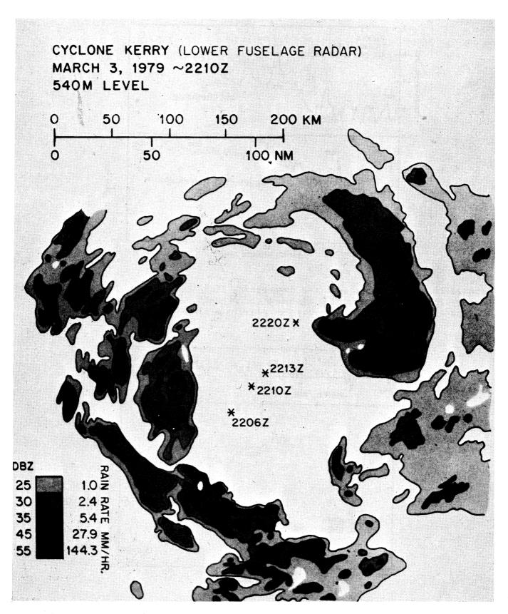
Figure 81. Digitized Plan Position Indicator radar depiction of Tropical Cyclone Kerry compositied from 2206 Z to 2220 Z on March 3, 1979.
