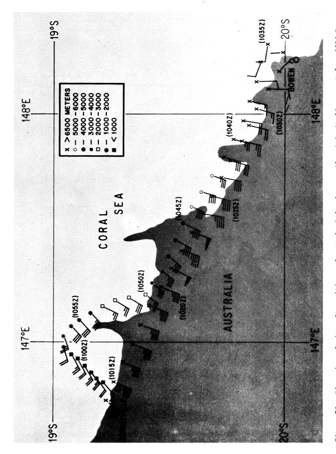
Figure 78. Plan view of aircraft position and actual winds along northeast Australian coast from 1014 Z to 1104 Z on March 1, 1979. (Altitudes of observations are indicated by symbols.)
