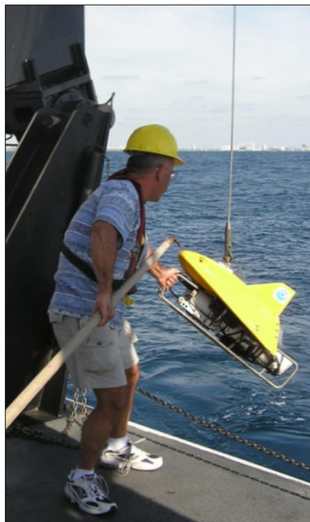
**Figure 17.** V-Fin instrument being deployed from the aft of the *RV Nancy Foster*.
