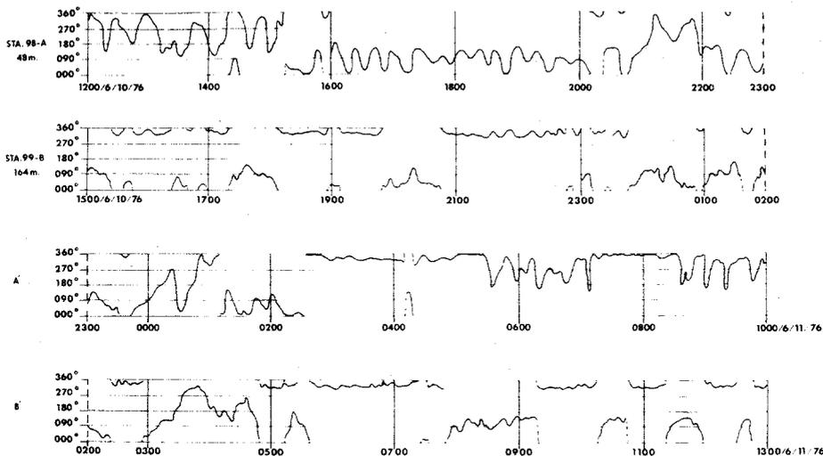
Fig. 3. Portion of current-meter records from Salt River Canyon showing the almost continuously changing directions at the depth of 48 m (3 m above the bottom) and the somewhat more constant up- and downcanyon direction at 164 m (also 3 m above the bottom). Note that two of the periods of downcanyon direction with fairly constant direction in the 48 m record may be matched about 3 hours later in the 164 m record.
