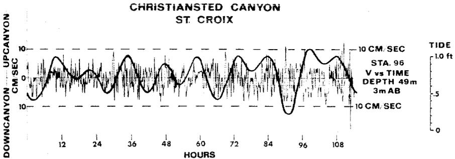
Fig. 4. Additional evidence of the effect of small tidal ranges in causing high frequency of up- and downcanyon currents at 49 m in Christiansted Canyon off St. Croix. Apparently there is no relationship between the currents and the tides, with the exception of a relatively strong downcanyon flow during falling tide near the end of the record.
