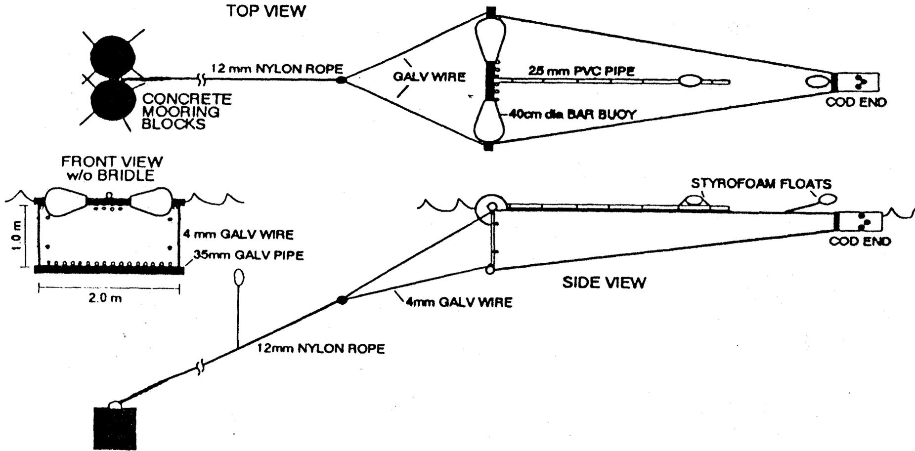
Figure 3. Schematic diagram of the surface and subsurface channel net and their mooring ( Shenker et al., 1993 ).
