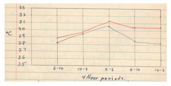
This gives a better picture of the water over air temperature. As in the first graph the red line represents water and the black air. Dotted lines are reversed for extremes (max. and min.).
