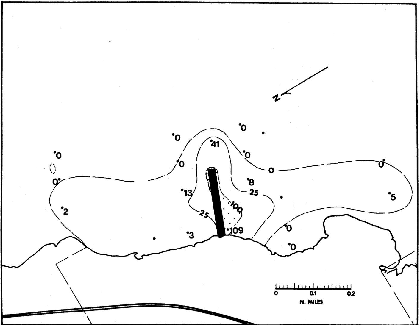
38 "Excess rates" attributable to the dredge project for the period January 15 to January 26, 1973 (Project days 85-96). The dredge was dormant, but erosion of the spoil by waves produced a zone of excess fallout exceeding  $>100 \text{ mg/cm}^2/\text{day}$  in the stippled area. See Figure 35 for an explanation of symbols.
