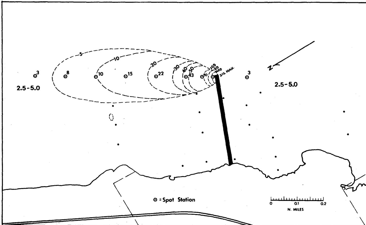
4 Dredge plume on May 30, 1973 (Project day 220) near the end of the active extension phase, with the turbidity diaper leaking badly. Both the maximum concentration (212 mg/l) and the maximum plume length (4038 feet) were observed at this time. The lateral boundaries of the plume are approximate, based on visual description; length and concentration are based on spot measurements at the points indicated.
