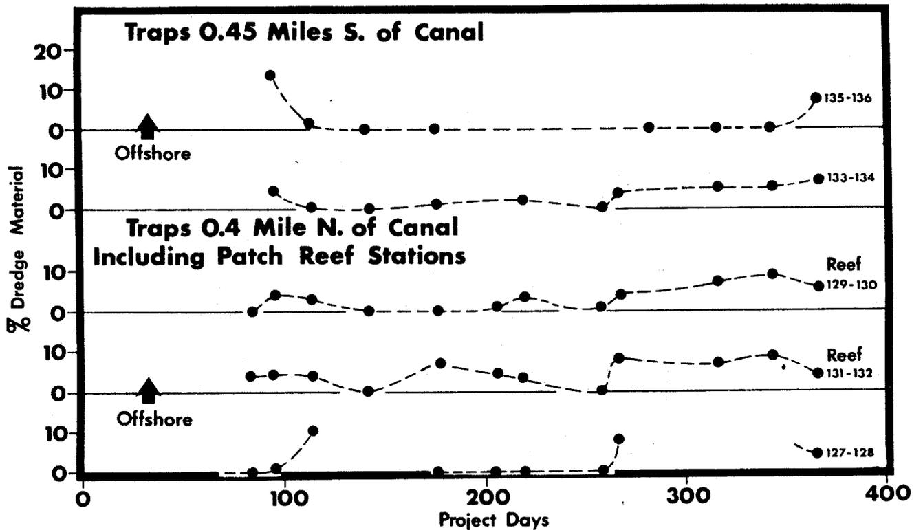
Percentage of dredge-derived sediment accumulated in traps along a line 0.45 n. mile south of the canal, and another line approximately 0.4 n. mile north of the canal, including the two stations nearest the coral patch reef. The percentages tended to increase toward the end of the project.
