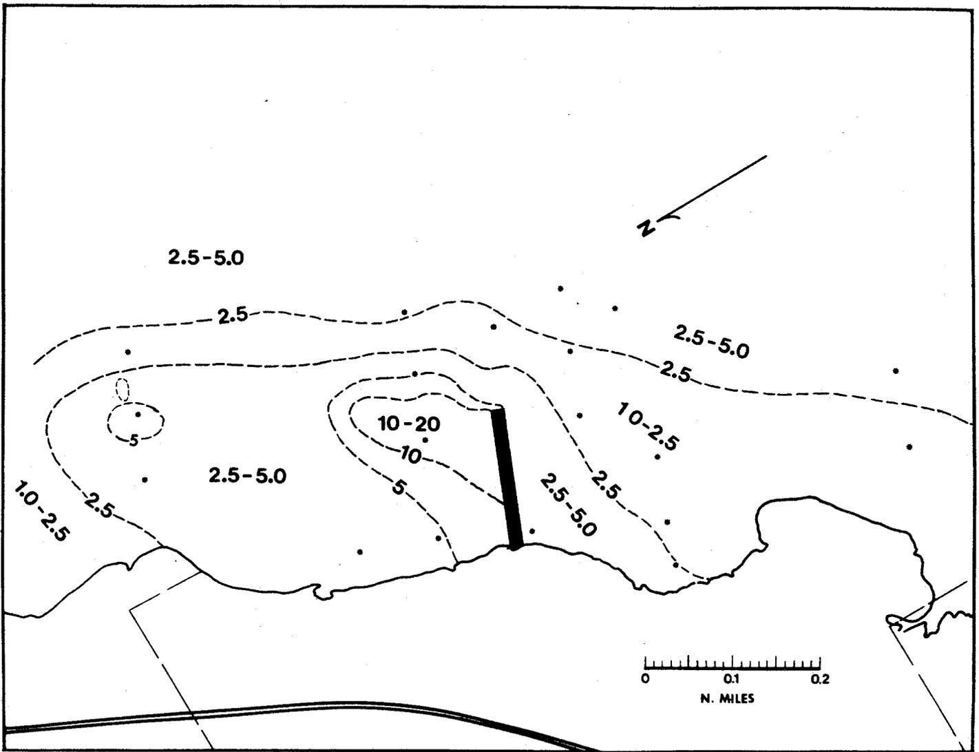
15b Concentration of suspended sediment in surface water on July 23, 1973 (Project day 274). Dredge was actively removing the spoil fingers, with a turbidity diaper.
