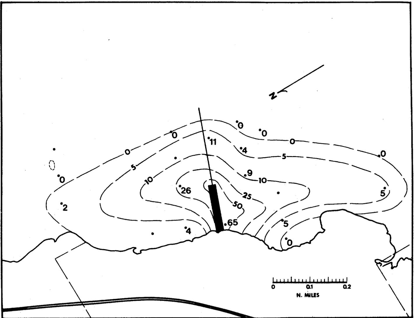
45 "Excess rates" attributable to the dredge project for the period July 9 to August 2, 1973 (Project days 260-284). The dredge, with a turbidity diaper, continued removing spoil. No excess was detected at the coral patch reef. See Figure 35 for an explanation of symbols.
