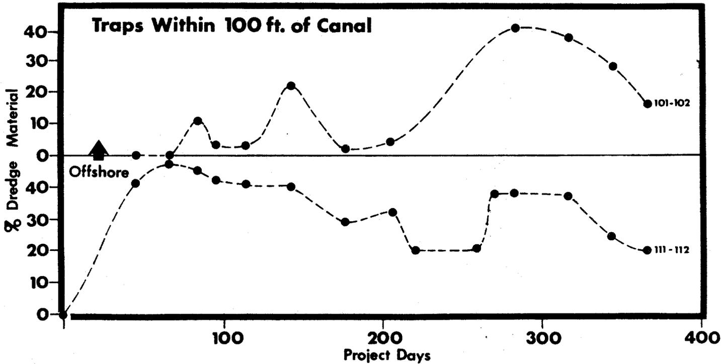
64 Percentage of dredge-derived sediment accumulated in traps within 100 feet of the canal, plotted as a function of project days, and compared with dredge activity. The most inshore trap (111-112) is plotted at the bottom of the figure. The percentage of dredge derived sediment reflected the proximity and activity of the dredge.
