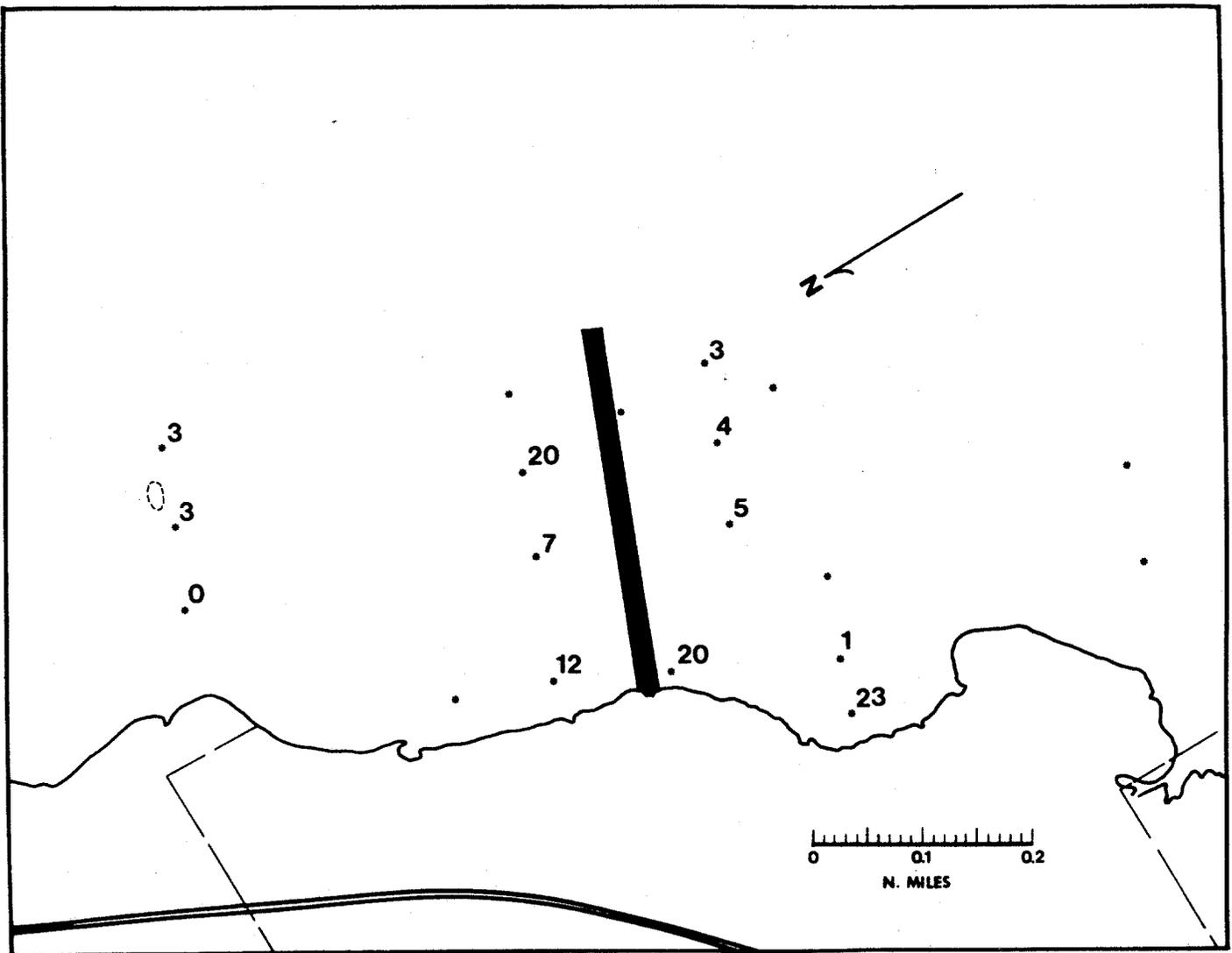
Percentage of dredge-derived sediment accumulated in sediment traps during the period May 11 to May 31, 1973 (Project days 201-221). The dredge resumed extending the canal about May 15 (day 205), now with a turbidity diaper for the first time, and reached its maximum extent approximately May 31 (day 231). On May 30 (day 230), the maximum plume concentration (212 mg/l) and maximum plume length were reached (Tables 2 and 3; Figures 4 and 5). See Figure 50 for an explanation of symbols.
