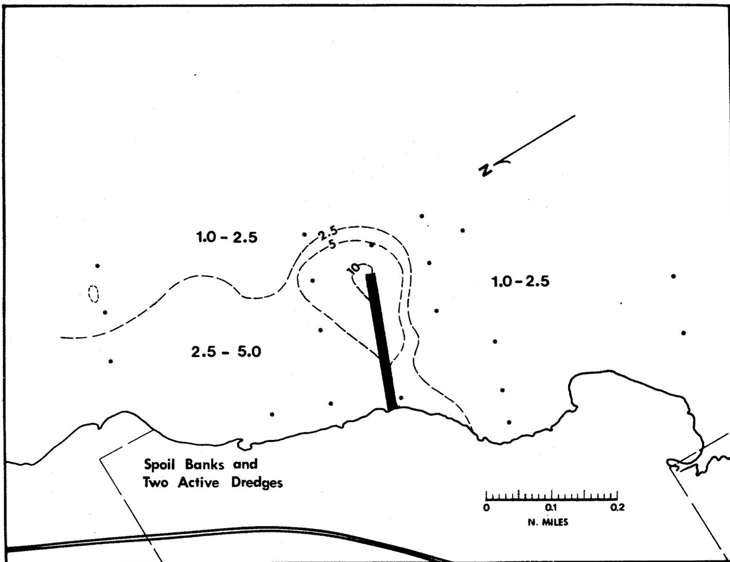
13b Concentration of suspended sediment in surface water on May 18, 1973 (Project day 208). Dredge was active, with a turbidity diaper for the first time.
