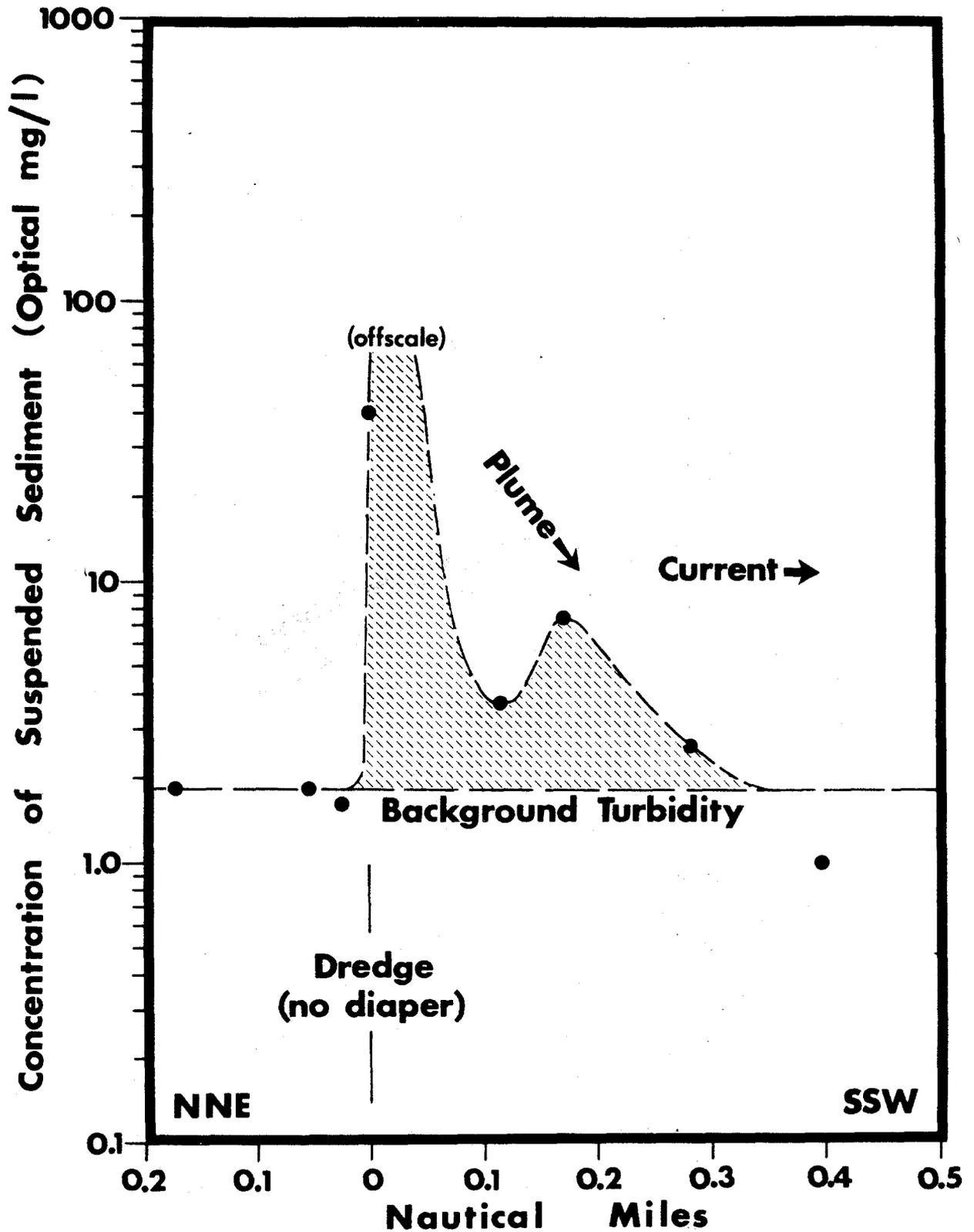
8c Concentration of suspended sediment in the most intense part of the plume vs distance from the dredge, November 16, 1972 (Project day 25). The maximum values were offscale on the 1-m transmissometer. Dredge was active, without turbidity diaper.
