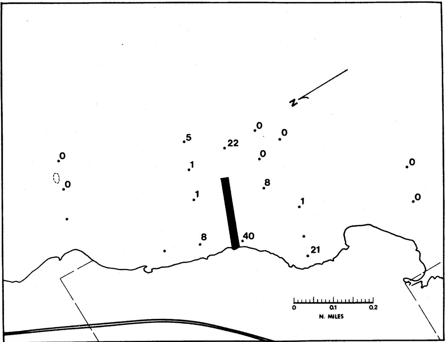
55 Percentage of dredge-derived sediment accumulated in sediment traps during the period February 14 to March 14, 1973 (Project days 115-143). The dredge was dormant, but waves continued to erode the spoil fingers. See Figure 50 for an explanation of symbols.
