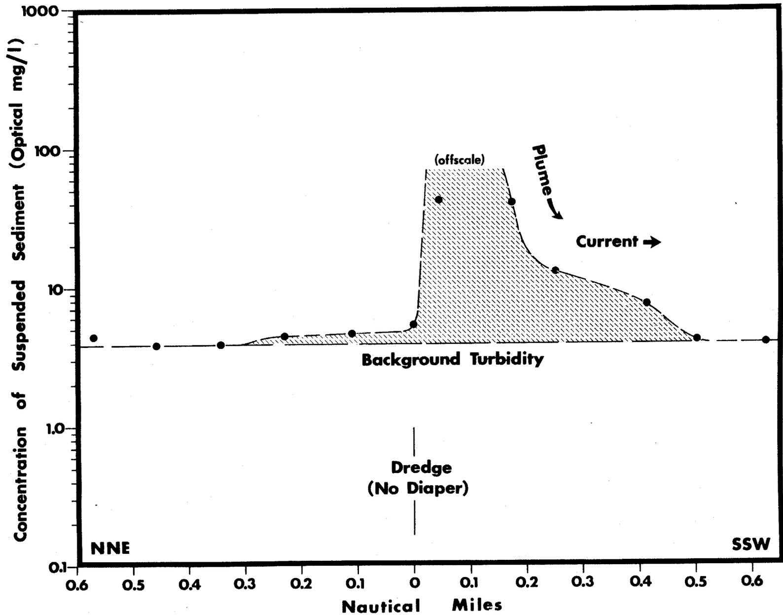
9c Concentration of suspended sediment in the most intense part of the plume vs distance from the dredge, December 11, 1972 (Project day 50). The maximum values were offscale on the 1-m transmissometer. Dredge was active, without turbidity diaper.
