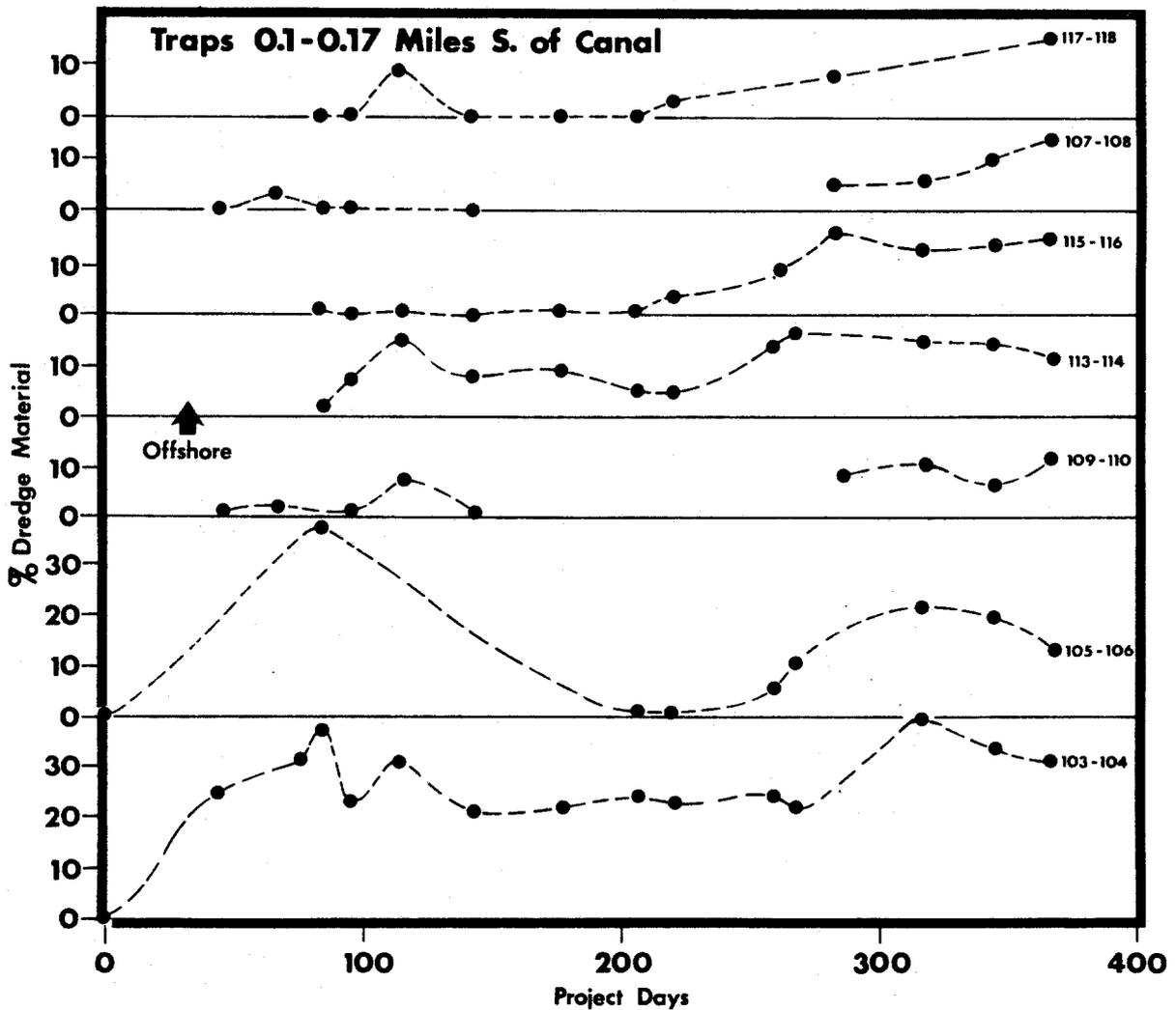
Percentage of dredge-derived sediment accumulated in traps along a line approximately 0.1-0.17 n. miles south of the canal. The percentages reflect the activity of the dredge and its proximity to the trap site.
