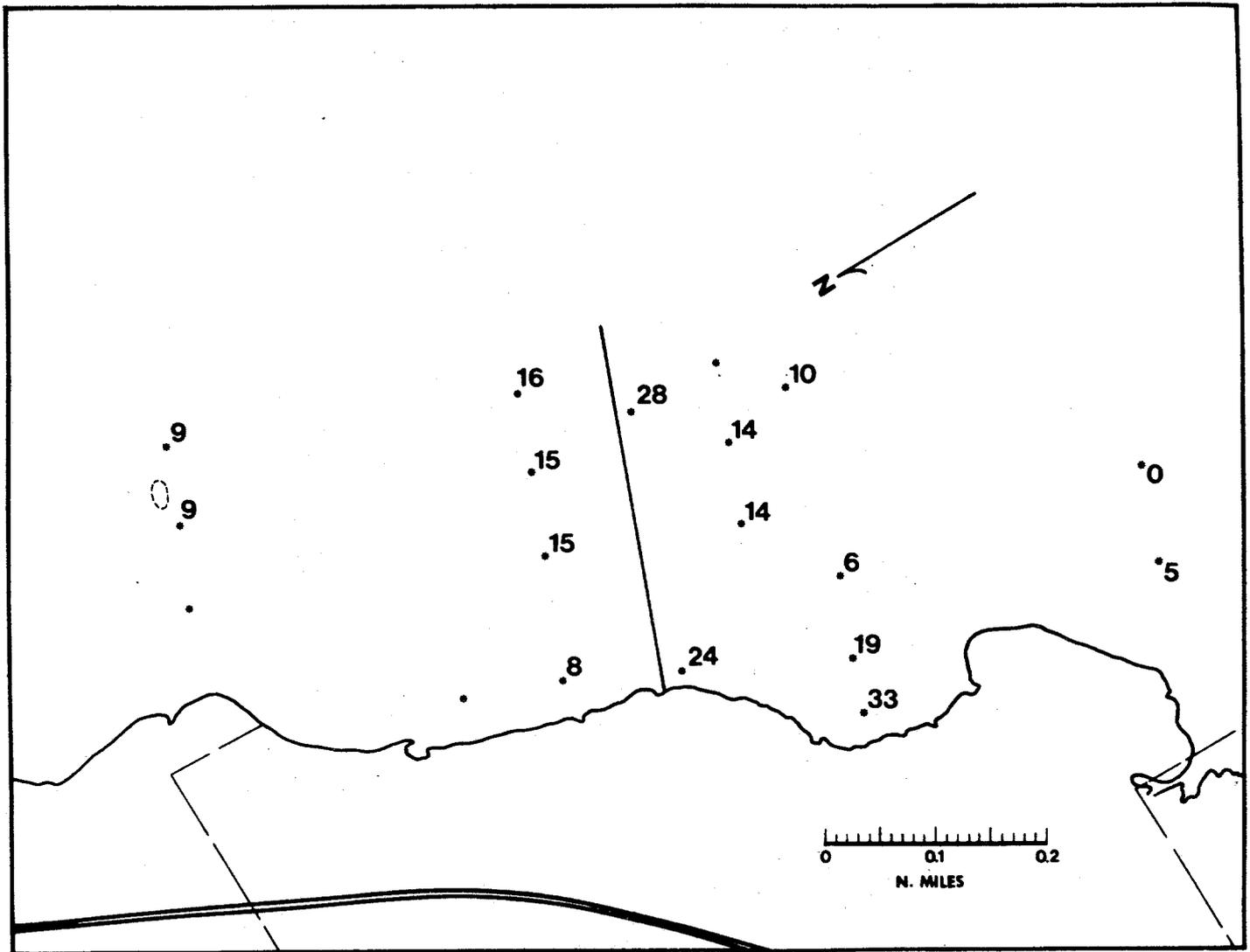
Percentage of dredge-derived sediment accumulated in sediment traps during the period September 5 to October 2, 1973 (Project days 318-345). Dredging was completed in the previous period (about day 300), so the dredge-derived sediment that continued to collect is residual, due to drainage of inland spoil, and possibly also to reworking of the bare bottom beneath the former spoil fingers, and to flushing of "canal fluff" from the canal axis. Symbols are explained on Figure 50.
