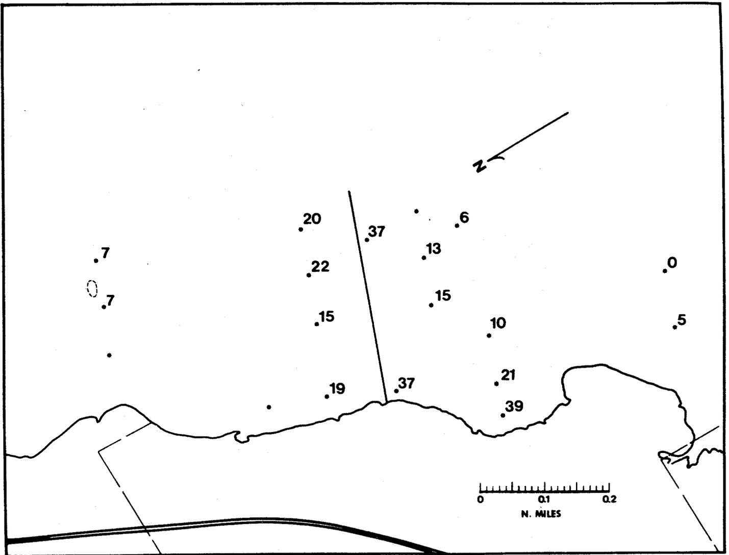
61 Percentage of dredge-derived sediment accumulated in sediment traps during the period August 2 to September 5, 1973 (Project days 284-318). The dredge completed removing the spoil fingers, and, although a turbidity diaper was in use, it leaked badly (cf. Figure 46). As with the previous period, traps near the canal axis collected large percentages of canal-derived debris. Symbols are explained on Figure 50.
