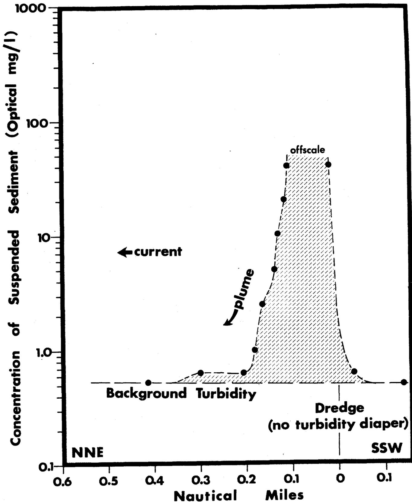
10c Concentration of suspended sediment in the most intense part of the plume vs distance from the dredge, December 26, 1972 (Project day 65). The maximum values were offscale on the 1-m transmissometer. Dredge was active, without turbidity diaper.
