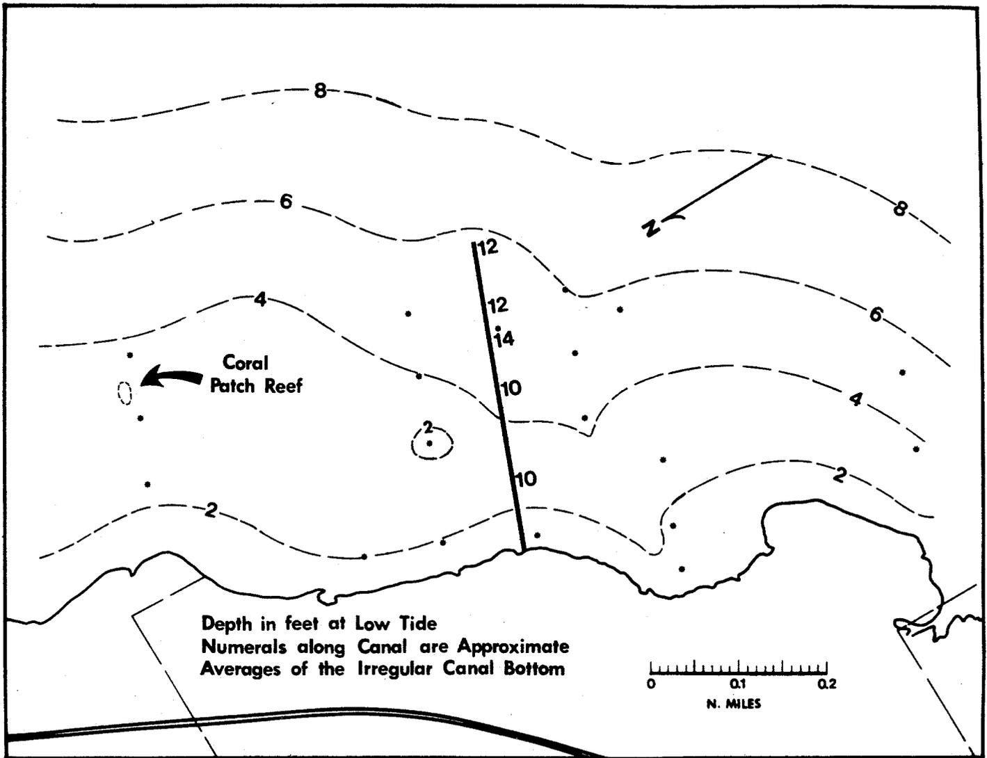
2 Bathymetry of the Basin Hills dredge site, also showing the axial depths of the completed canal, and the coral patch reef used as a biological indicator. Depths in feet at low tide.
