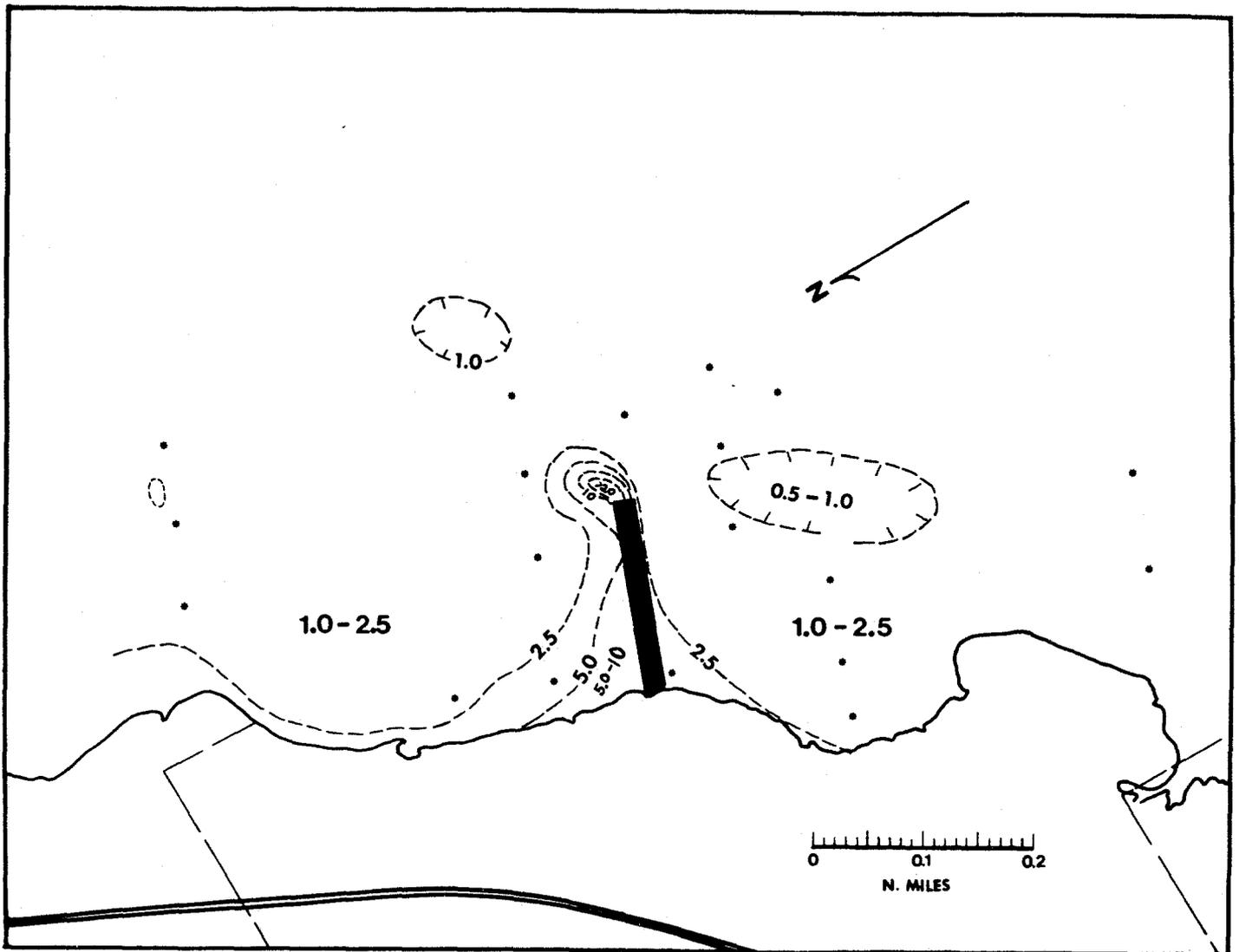
12b Concentration of suspended sediment in surface water on May 14, 1973 (Project day 204). The dredge had been inactive for the previous 134 days, and the spoil fingers were being eroded by waves.
