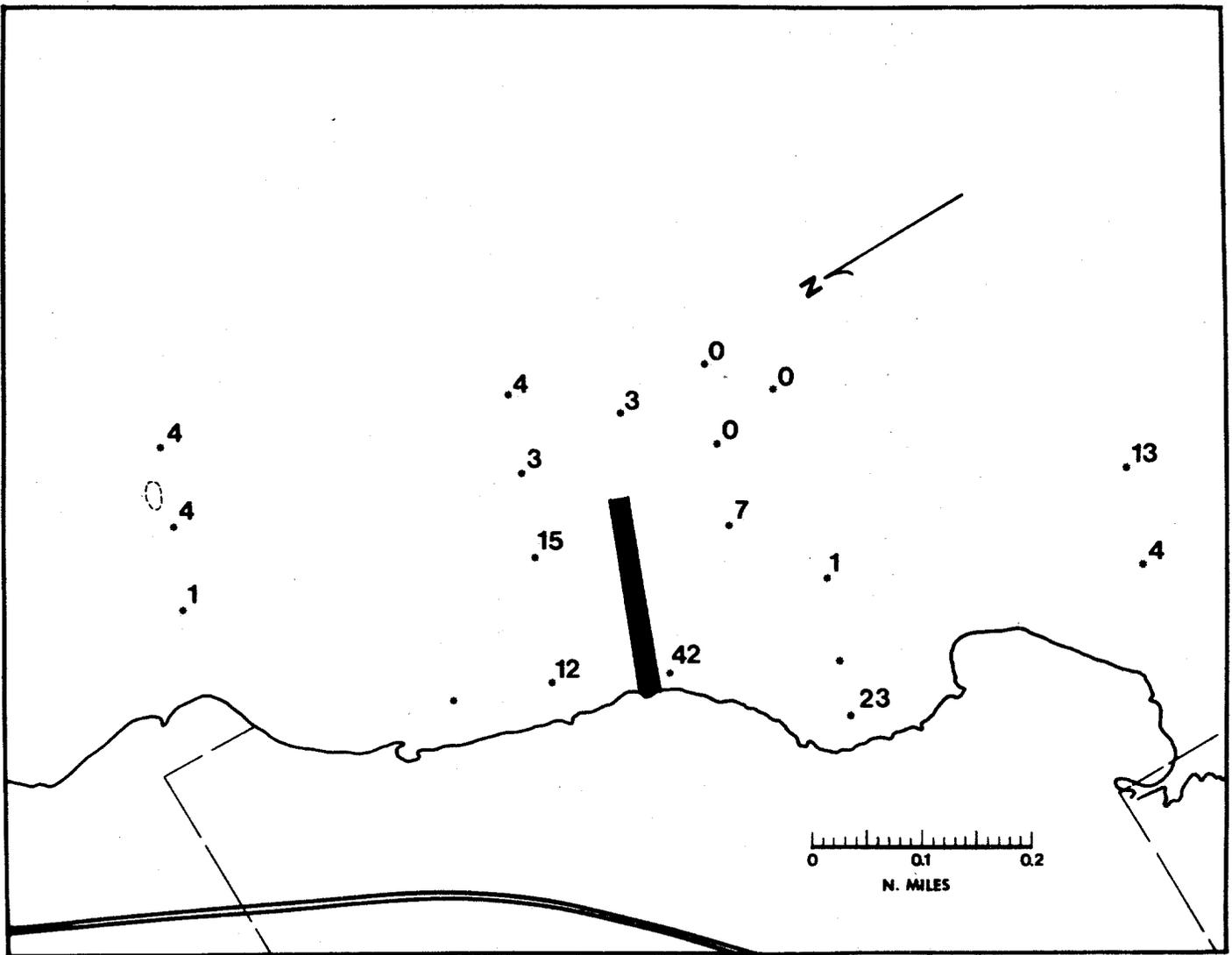
Percentage of dredge-derived sediment accumulated in sediment traps during the period January 15 to January 26, 1973 (Project days 85-96). The dredge was dormant, but the spoil fingers were being eroded by waves. See Figure 50 for an explanation of symbols.
