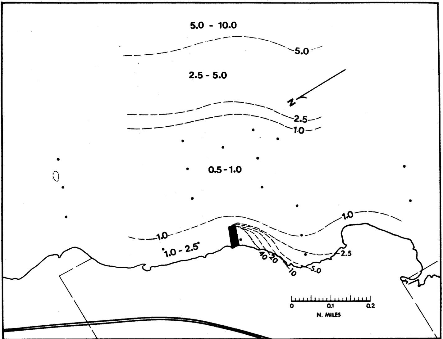
8b Concentration of suspended sediment in surface water on November 16, 1972 (Project day 25). Dredge was active, without turbidity diaper.
