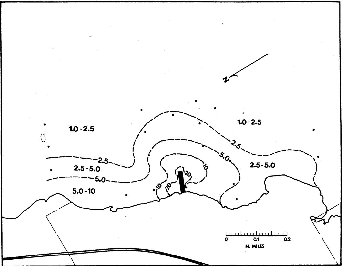
16b Concentration of suspended sediment in surface water on August 7, 1973 (Project day 289). Dredge was actively removing the spoil fingers, with a turbidity diaper.
