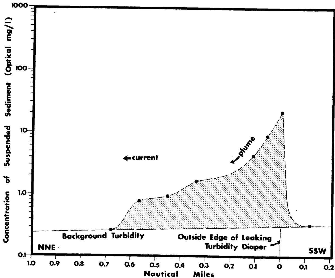
5 Concentration of suspended sediment in the most intense part of the plume vs distance from the dredge on May 30, 1973 (Project day 220). Dredge was actively extending the spoil fingers, with a turbidity diaper in place but leaking badly. Both the maximum concentration (212 mg/l) and the maximum plume length (4038 feet) were observed at this time.
