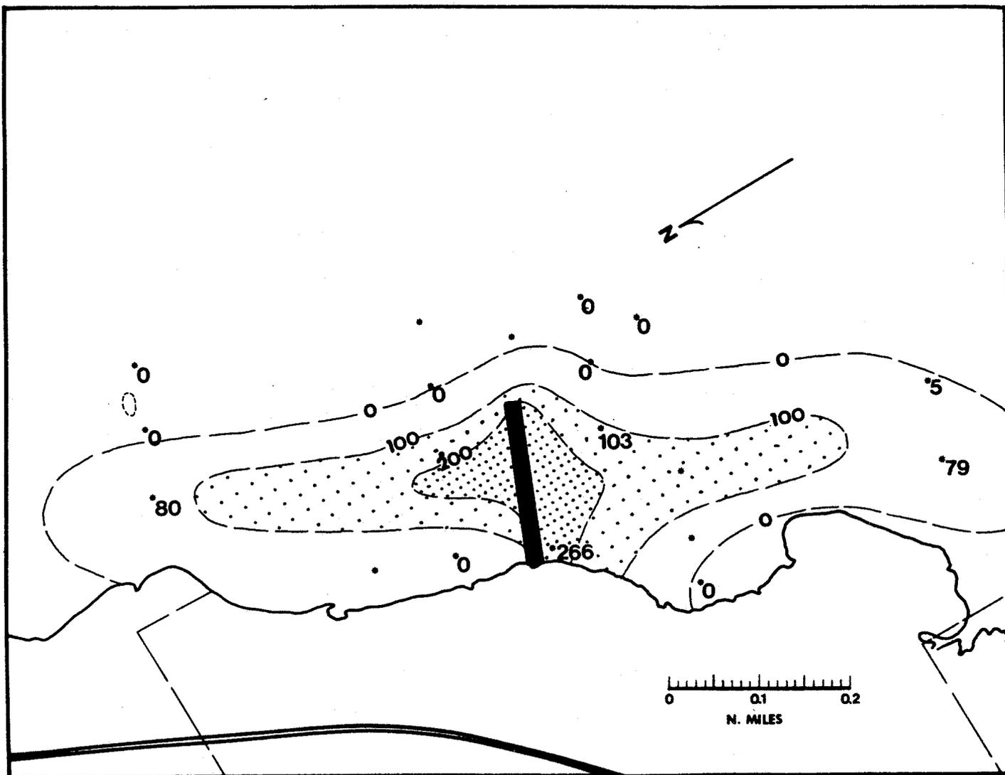
41 "Excess rates" attributable to the dredge project for the period March 14 to April 18, 1973 (Project days 143-178). The dredge was dormant, but continued erosion of the spoil by waves produced a relatively intense fallout zone as indicated by stippling. See Figure 35 for an explanation of symbols.
