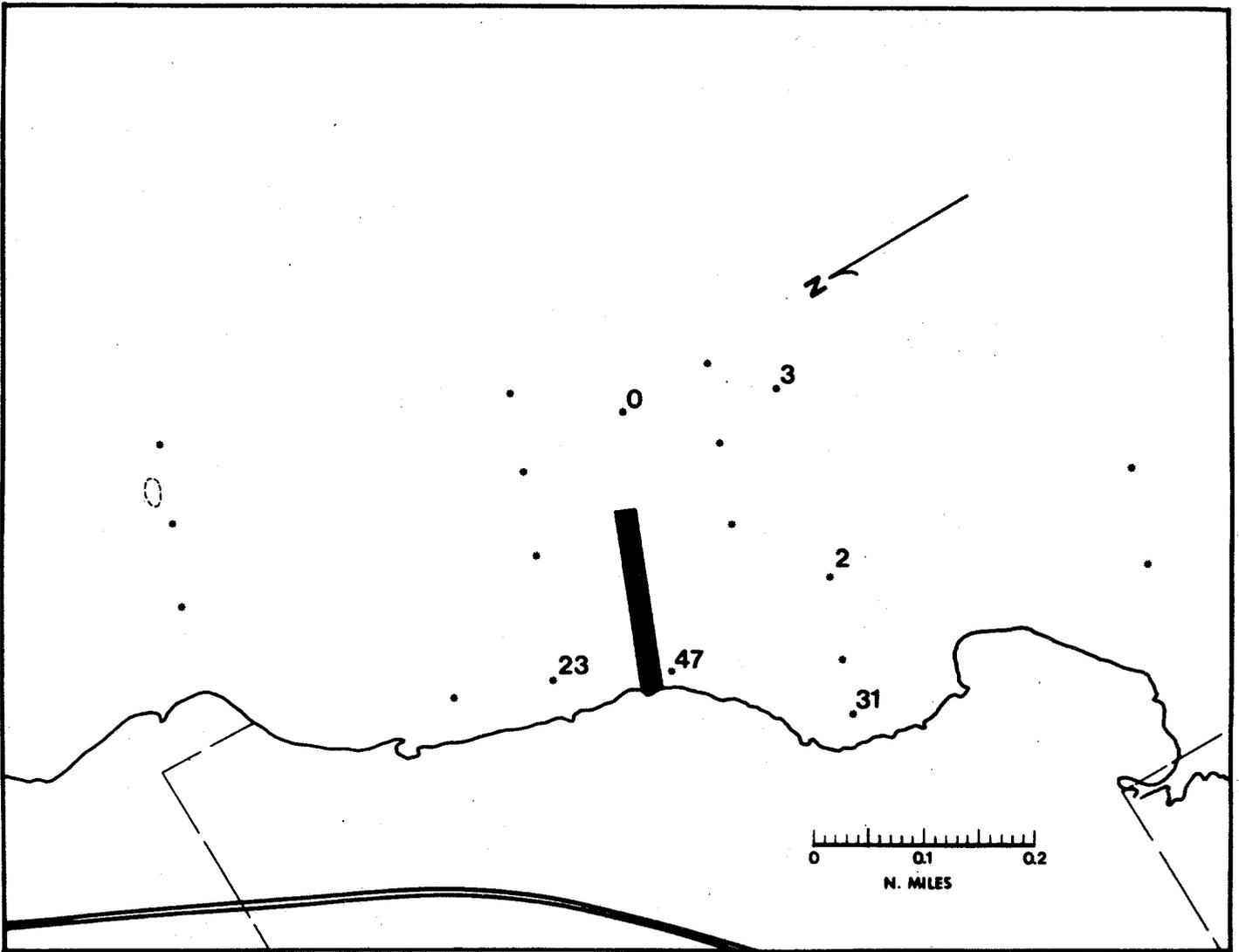
51 Percentage of dredge-derived sediment accumulated in sediment traps during the period December 7 to December 28, 1972 (Project days 46-67). The dredge was actively extending the canal, without a turbidity diaper. See Figure 50 for an explanation of symbols.
