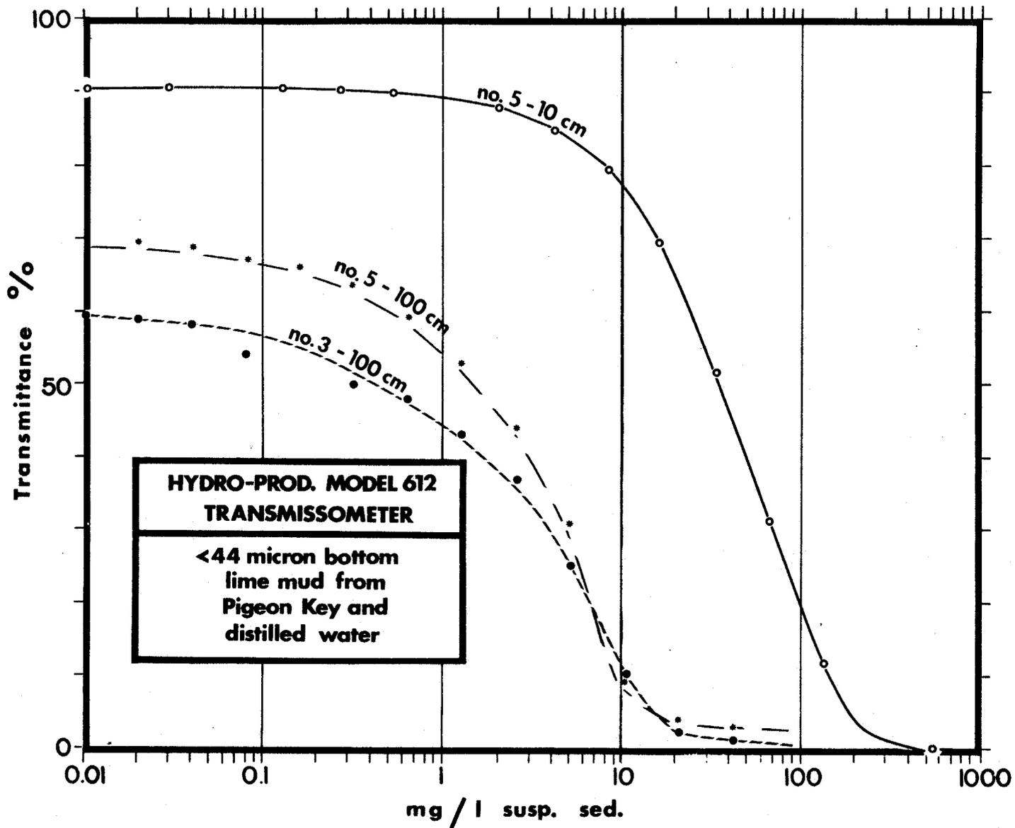
6 Working curve of light transmittance (%) versus suspended sediment concentration (mg/l) for path lengths of 10 cm and 100 cm. Determined in a laboratory test tank with two Hydro-Products Model 612 transmissometers (our No. 3 and No. 5), distilled water, and known weights of salt-free, <44 micron  $\text{CaCO}_3$  mud from a shoal 100 yd. west of the U. of Miami marine station on Pigeon Key.
