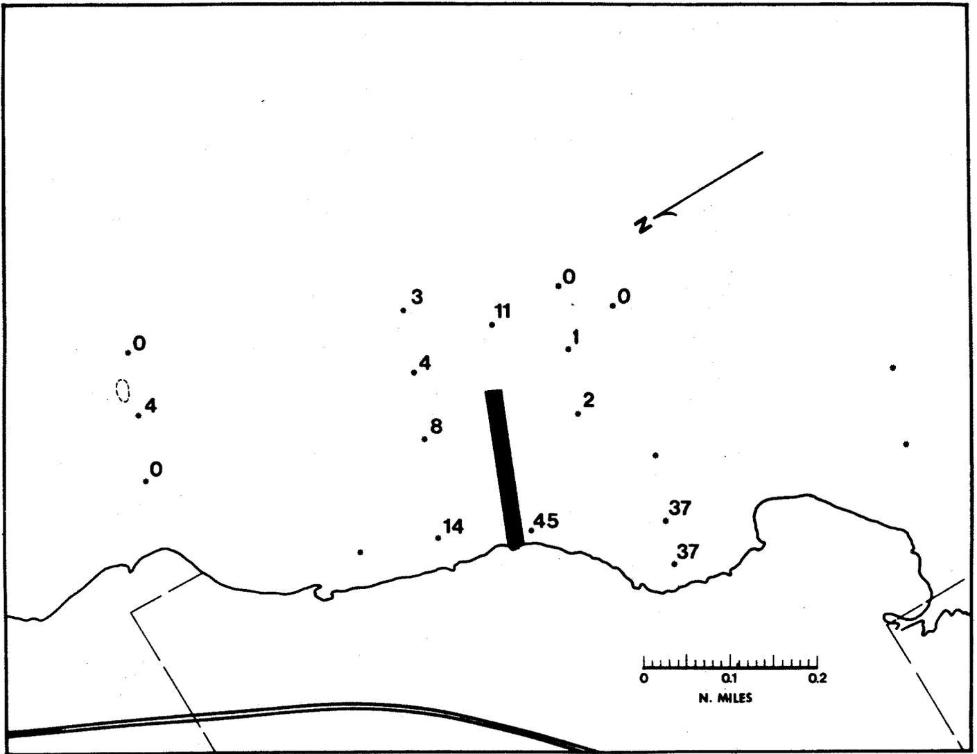
Percentage of dredge-derived sediment accumulated in sediment traps during the period December 28, 1972 to January 15, 1973 (Project days 67-85). The dredge was active only until December 31, after which it plugged the canal end and withdrew for 4 1/2 months. Most of the dredge effluent moved northward; about 4% of the sediment reaching the coral patch reef was of dredge origin. See Figure 50 for an explanation of symbols.
