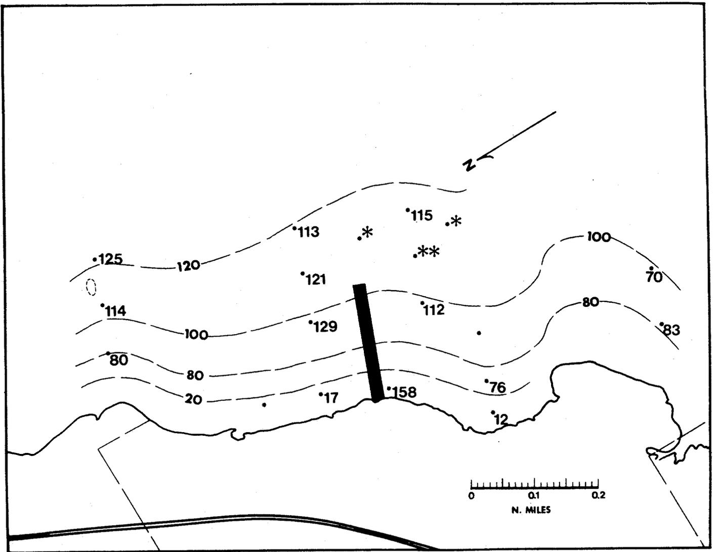
25 "Total rates" and "natural rates" of accumulation for the period January 26 to February 14, 1973 (Project days 96-115). An unusually severe cold front caused the abnormally high accumulation rates.
