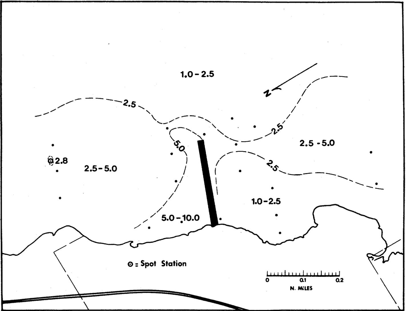
14b Concentration of suspended sediment in surface water on July 11, 1973 (Project day 262). Dredge was actively removing the spoil fingers, with a turbidity diaper.
