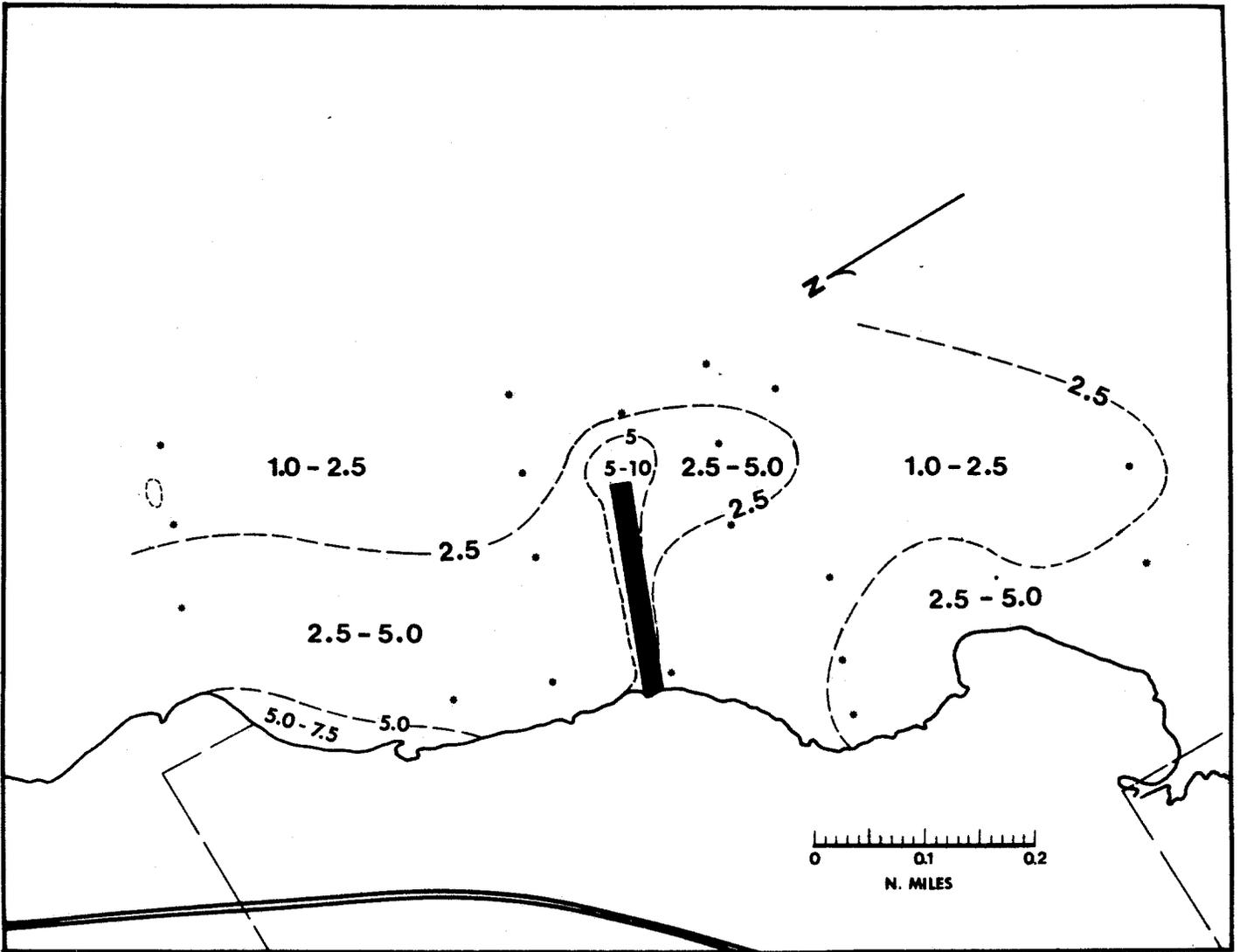
11b Concentration of suspended sediment in surface water on March 22, 1973 (Project day 151). The dredge had been inactive for the previous 81 days, and the spoil fingers were being eroded by waves.
