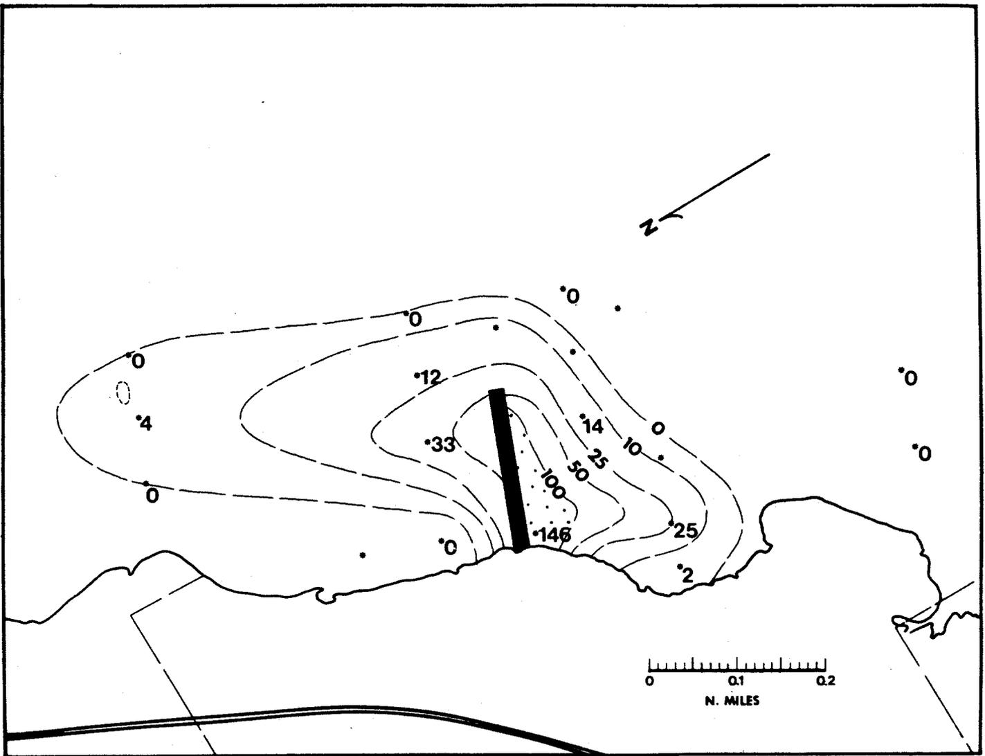
39 "Excess rates" attributable to the dredge project for the period January 26 to February 14, 1973 (Project days 96-115). The dredge was dormant, but continued erosion of the spoil by waves, accelerated by a severe cold front, produced a zone of excess fallout, exceeding  $>100 \text{ mg/cm}^2/\text{day}$  in the stippled area. A very small amount of excess sediment ( $4 \text{ mg/cm}^2/\text{day}$ ) reached the coral patch reef. See Figure 35 for an explanation of symbols.
