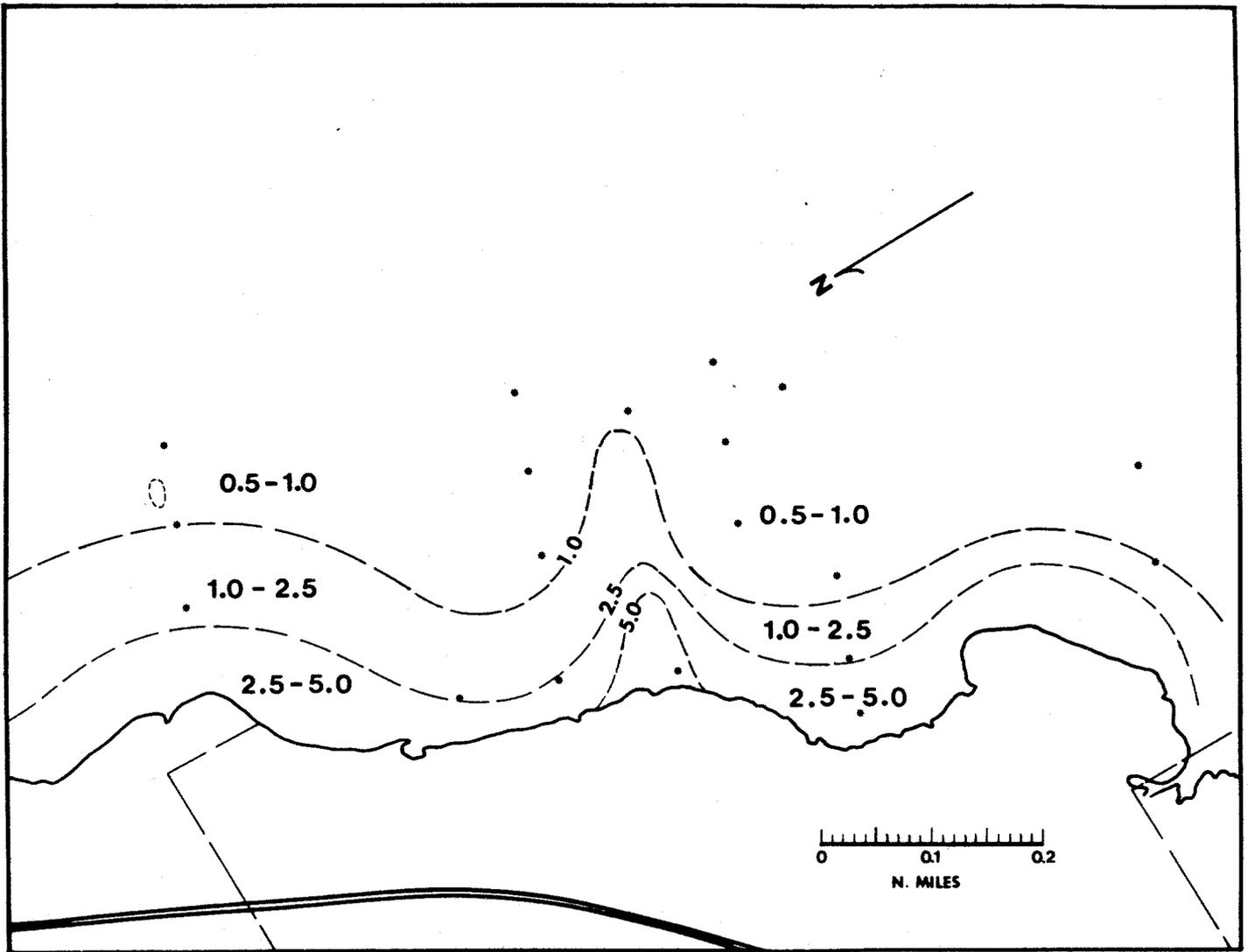
18b Concentration of suspended sediment in surface water on September 13, 1973 (Project day 326). Dredging had been completed approximately 30 days earlier, but some residual turbidity remains near the canal.
