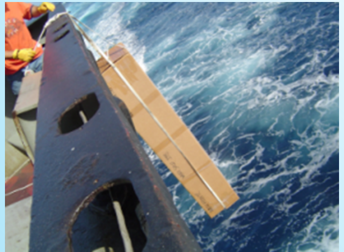
Argo float being deployed by an AOML technician from the Horizon Hawaii
