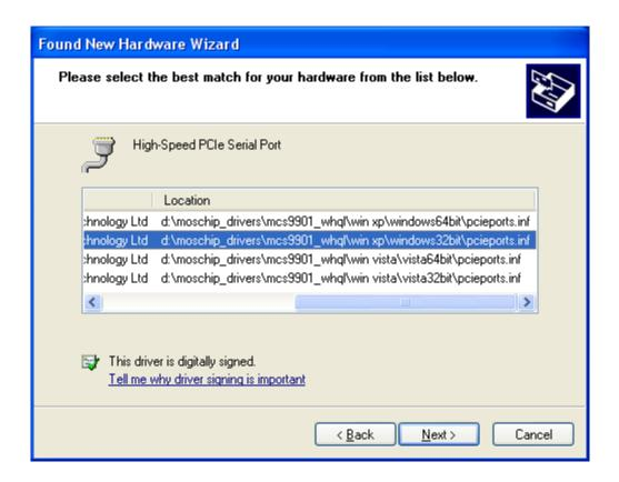
After installation you will find two new PCIe Serial Ports a PCIe parallel port added to your system hardware. Currently only the first serial port is actually used, the other two ports are currently reserved for future use. Please do not try to manually change these port characteristics.
