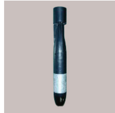
FIGURE 1-12: XCTD Probe
