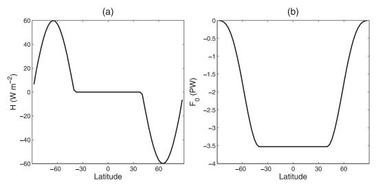
FIG. 1. (a) Latitudinal distribution of imposed oceanic fluxes  $(H, \text{ in W m}^{-2})$  and (b) associated implied meridional oceanic heat transport  $(F_0, \text{ in PW})$  with  $H = -1/(2\pi a^2 \cos\phi) \partial F_0/\partial \phi$  when  $A = 60 \text{ W m}^{-2}$ .
