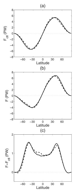
FIG. 9. The vertically integrated moist static energy transports F (PW) for (a) A = 0 W m<sup>-2</sup> and (b) A = 60 W m<sup>-2</sup>, and (c) the anomalous vertically integrated moist static energy transports,  $F - F_{\rm ctl}$  (PW) for A = 60 W m<sup>-2</sup> in the simplified moist GCM (solid line) and the energy balance model (dashed line).
