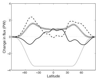
FIG. 4. The change in vertically integrated moist static energy transports,  $F-F_{\rm ctl}$  (in PW, solid line with circles), the anomalous mean energy transports (solid line), the anomalous eddy energy transports (dashed line), and the imposed oceanic flux,  $F_0$  (gray line) for  $A=60~{\rm W~m^{-2}}$ .
