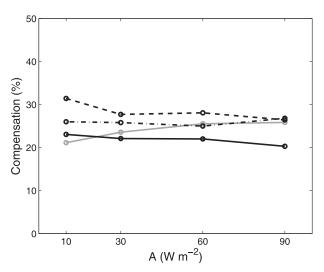
FIG. 5. The fraction of the imposed forcing that is balanced by the atmospheric energy flux averaged over  $20^{\circ}$ S and  $20^{\circ}$ N (C in %) as a function of the strength of forcing A for the idealized GCM with RH<sub>SBM</sub> = 70% (gray solid line), RH<sub>SBM</sub> = 85% (black dashed line), and RH<sub>SBM</sub> = 100% (black solid line), and the energy balance model (black dashed–dotted line).
