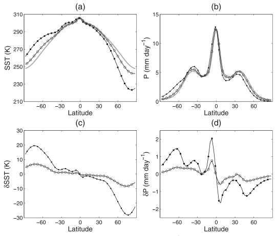
FIG. 2. Time mean, zonal mean (a) SST (K), (b) precipitation (mm day<sup>-1</sup>), (c) the change in SST (K), and (d) the change in precipitation (mm day<sup>-1</sup>) for A = 0 W m<sup>-2</sup> (gray line), A = 30 W m<sup>-2</sup> (black line with circles), and A = 90 W m<sup>-2</sup> (black line with squares) where A is the amplitude of the imposed forcing H.
