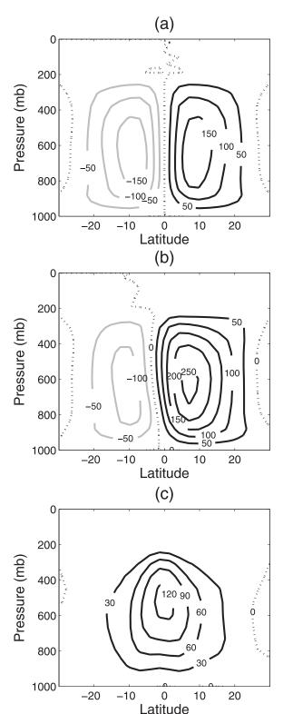
FIG. 3. Time mean, zonal mean streamfunction (in  $10^9$  kg s<sup>-1</sup>) for (a) the control case A=0 W m<sup>-2</sup> and (b) A=60 W m<sup>-2</sup>. (c) The change in time mean, zonal mean streamfunction for A=60 W m<sup>-2</sup>. Black (gray) contours correspond to clockwise (counterclockwise) circulation.
