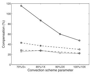
FIG. 15. Here, C (%) by the atmospheric energy flux averaged over 20°S and 20°N as a function of a convection scheme parameter (RH<sub>SBM</sub> in the simplified moist GCM and Tokioka parameter  $\alpha$  in AM2). Gray (black) solid line indicates the simplified moist GCM (AM2), and dashed (dashed–dotted) line indicates AM2 with prescribed clouds (and water vapor).
