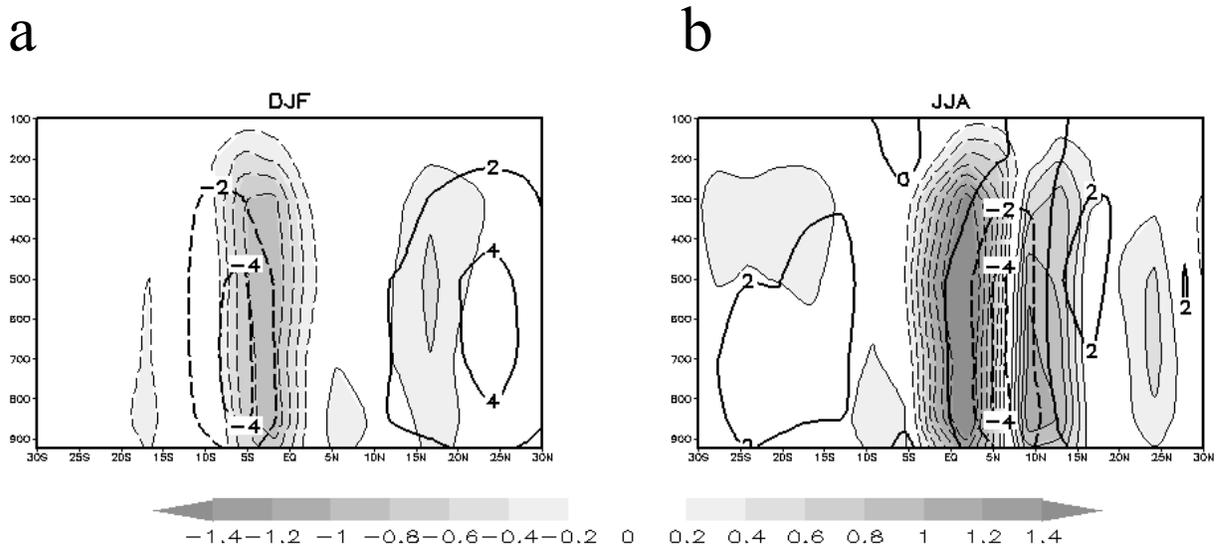
Fig. 4 a. Omega in  $\text{hPa s}^{-1}$  averaged over ( $50^\circ\text{W} - 25^\circ\text{E}$ ) for DJF. Thick contour lines: CONTROL run. Dashed lines indicate negative values (upward motion), the zero contour is omitted; Shaded: Difference between NO-THC and CONTROL run. b. As (a) but for JJA.
