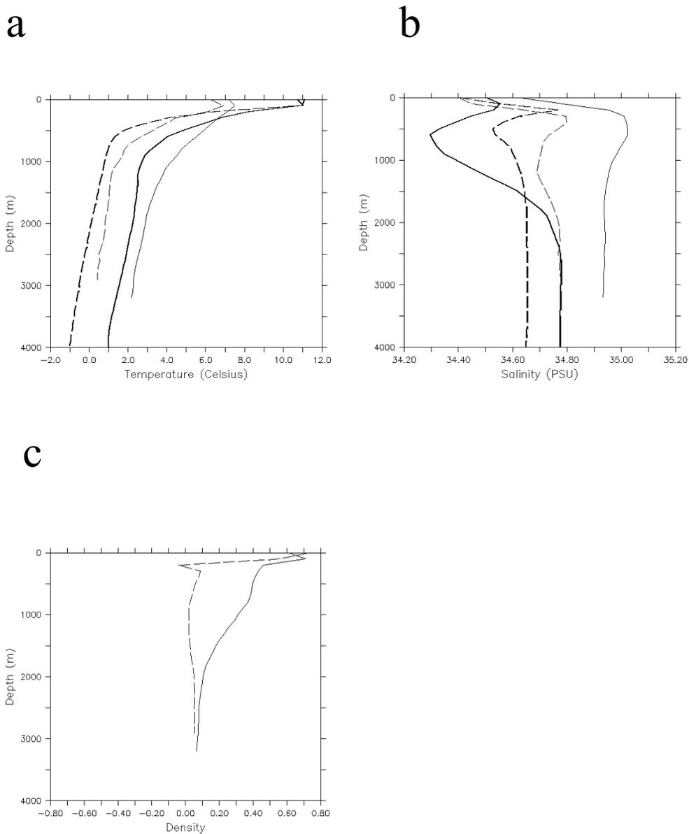
Fig.2 a. Zonal mean temperature ( $^{\circ}\text{C}$ ) profiles of the lateral boundaries in MICOM. Solid lines CONTROL run, dashed lines NO-THC run. Thin lines northern boundary, thick lines southern boundary; b. As (a) but now for salinity (PSU); c. Zonally mean averaged difference in density ( $\sigma_{\theta}$ ) between the northern and southern boundary for the CONTROL run (solid) and the NO-THC run (dashed).
