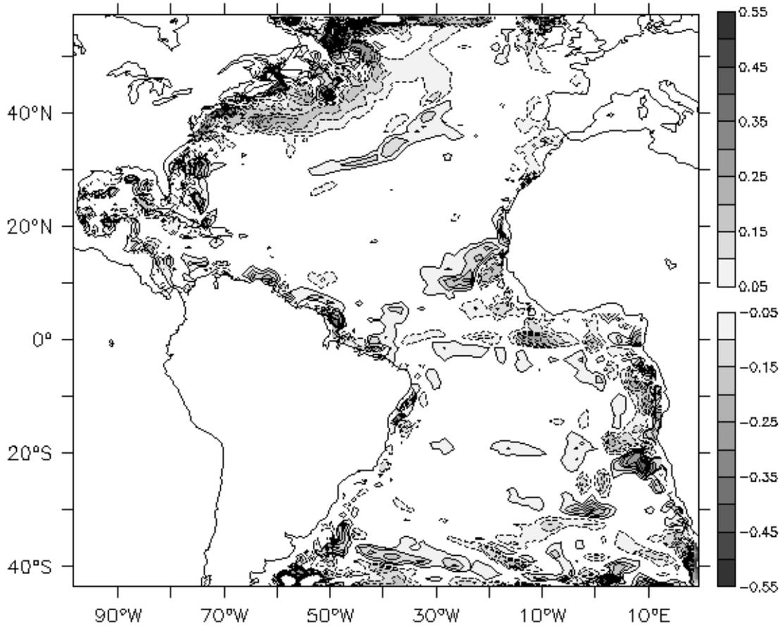
Fig. 6 a. Contribution of the ocean heat transport to the change between NO-THC and CONTROL in the heat budget of the mixed layer in  $10^{-6} \text{ K s}^{-1}$ . Dashed contours indicate negative values, the zero contour is omitted; b. As (a) but now only for the vertical ocean heat transport, i.e entrainment; c. As (a) but now only for the horizontal heat transport.
