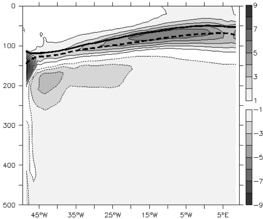
Fig. 8. Cross-section along the equator of the temperature difference ( $^{\circ}\text{C}$ ) between the CONTROL and NO-THC run. Dashed contours indicate negative values, the zero contour is omitted. The thick solid and dashed lines indicate the depth of the  $20^{\circ}\text{C}$  isotherm for the CONTROL and NO-THC run respectively.
