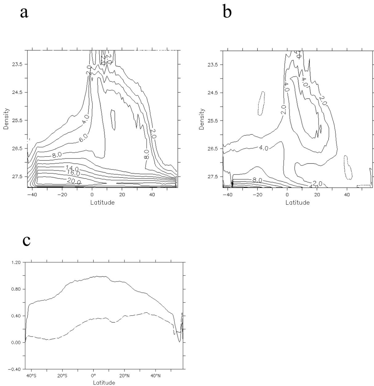
Fig. 7 a. Meridional overturning circulation in Sv for the CONTROL run; b. As (a) but for the NO-THC run; c: Meridional heat transport in PW for the CONTROL (solid line) and NO-THC experiment (dashed line).
