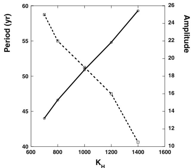
**Fig. 11** Dependence of period (in years, *solid*) and amplitude of the maximum meridional overturning streamfunction (in sverdrup, *dashed*) of the multidecadal finite amplitude oscillation on  $K_H$  for the MOM configuration as in Fig. 9
