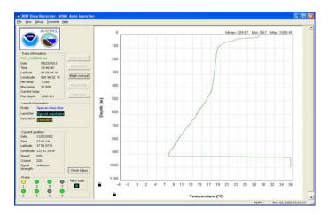
Fully automatic, the application is able to determine if tubes in the launcher are empty as well as diagnose several issues with the probe before and during the deployment. Bad deployments can be repeated automatically and tubes skipped in case of missing probes.
