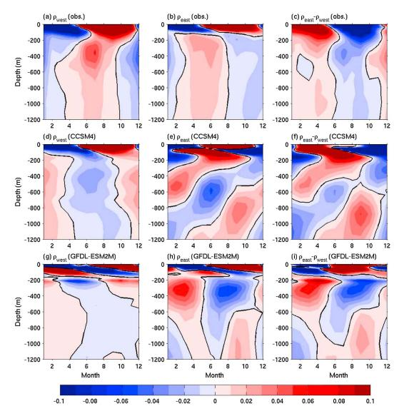
**Figure 3.** Water density at the (a) western and (b) eastern boundaries and (c) their differences (east minus west) from Argo climatology. (d–f) The same as Figures 3a–3c but from CCSM4 and (g–i) are from GFDL-ESM2M. As for Figure 2, the time-mean values at each depth have been removed. Units are in kg/m<sup>3</sup>.
