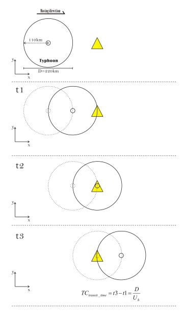
Fig. 3: Schematic diagram illustrating the situation as typhoon approaches a point location in ocean, as simulated by the 1-D mixed layer model. The inner core diameter (D) used in this work is 220km and the TC\_transit time is calculated as D/Uh.
