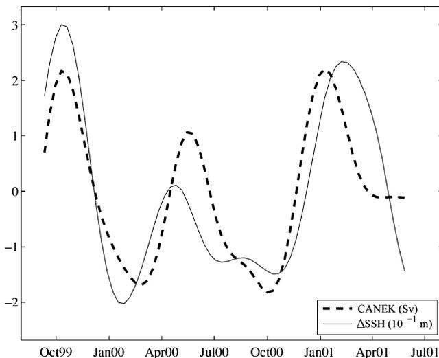
**Fig. 4** The index ( $\Delta$ SSH, *solid line*) calculated from the sea surface height anomaly difference, location B minus location A, shown in Fig. 3b, based on the Topex/Poseidon sea surface height anomaly measurement (low-pass filtered with a cut-off time scale of 120 days). The *dashed line* represents transport anomaly estimates from CANEK (low-pass filtered with a cut-off time scale of 120 days) for the Yucatan Channel from September 1999 to May 2001, referenced to the long-term mean
