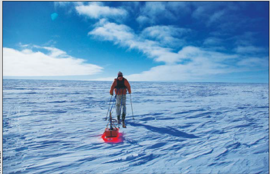
A scientist takes radar measurements to detect liquid water stored within the Greenland Ice Sheet in April 2013.
