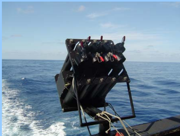
Autolauncher installed on the Horizon Hawaii
