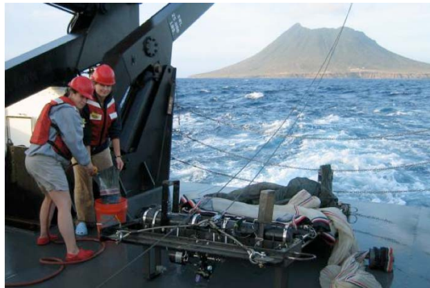
Scientists aboard the NOAA Ship Nancy Foster preparing to deploy a multiple opening and closing net, with an environmental sensing system (MOCNESS) in the northeastern Caribbean off the island of Saint Eustachius.
