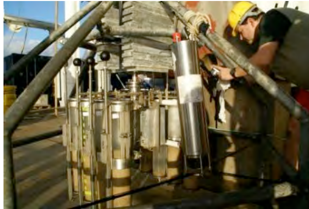
Figure 51 Oktopus Gmbh multiple corer (head version MUC 8/100) equipped with 8 transparent polycarbonate cylinders deployed during the BONUS-GOODHOPE cruise
