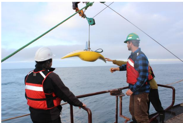
Botwing multi-frequency biomass sonar being deployed separated from the MOCNESS for a transect of the bloom
