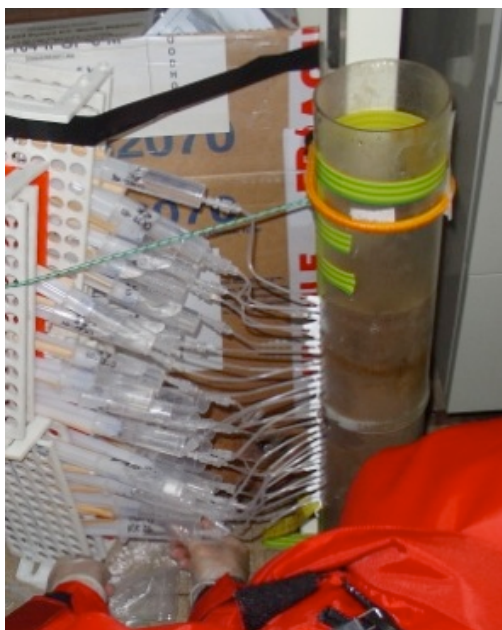
Figure 52 In situ filtration with Rhizon® (porous probes, 0.2 μm)
