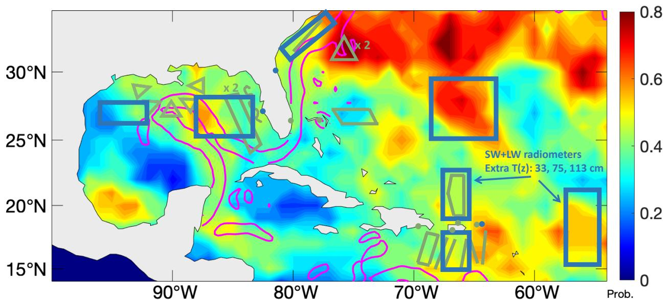
**Figure 1** Planned 2022 saildrone operational domains (blue boxes). Also shown are planned underwater glider tracks (green lines), saildrone deployment locations (blue dots), and glider deployment locations (green dots). Colored shading indicates probability of tropical storm-force winds during August-October, based on tropical cyclone data during 2000-2019. Pink contour line indicates surface currents of  $50 \text{ cm s}^{-1}$  on September 15, 2021.
