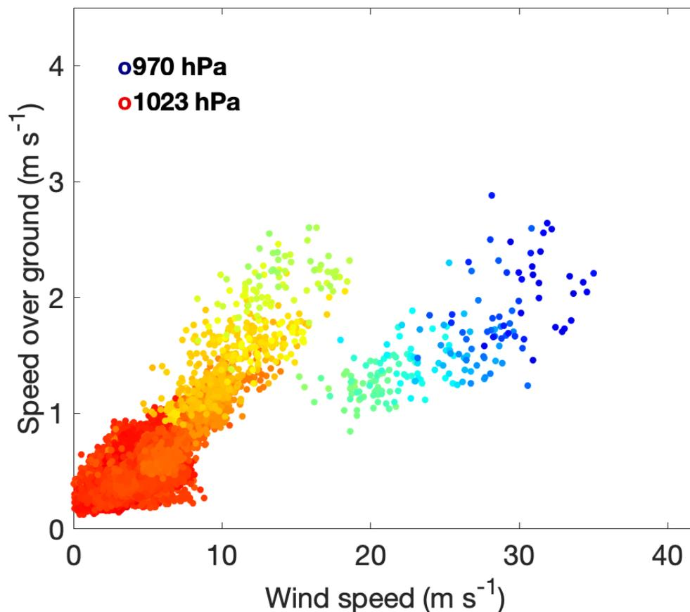
**Figure 13** Scatterplot of SD-1078's speed over ground vs. measured 1-min. wind speed for the duration of its mission, color-coded by measured barometric pressure (rainbow palette with extremes shown in legend).
