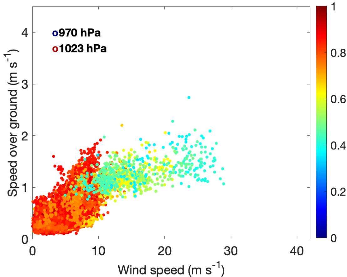
**Figure 17** Scatterplot of SD-1059's speed over ground vs. measured 1-min. wind speed for the duration of its mission, color-coded by measured barometric pressure (rainbow palette with extremes shown in legend).
