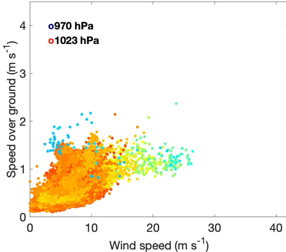
**Figure 9** Scatterplot of SD-1031's speed over ground vs. measured 1-min. wind speed for the duration of its mission, color-coded by measured barometric pressure (rainbow palette with extremes shown in legend).
