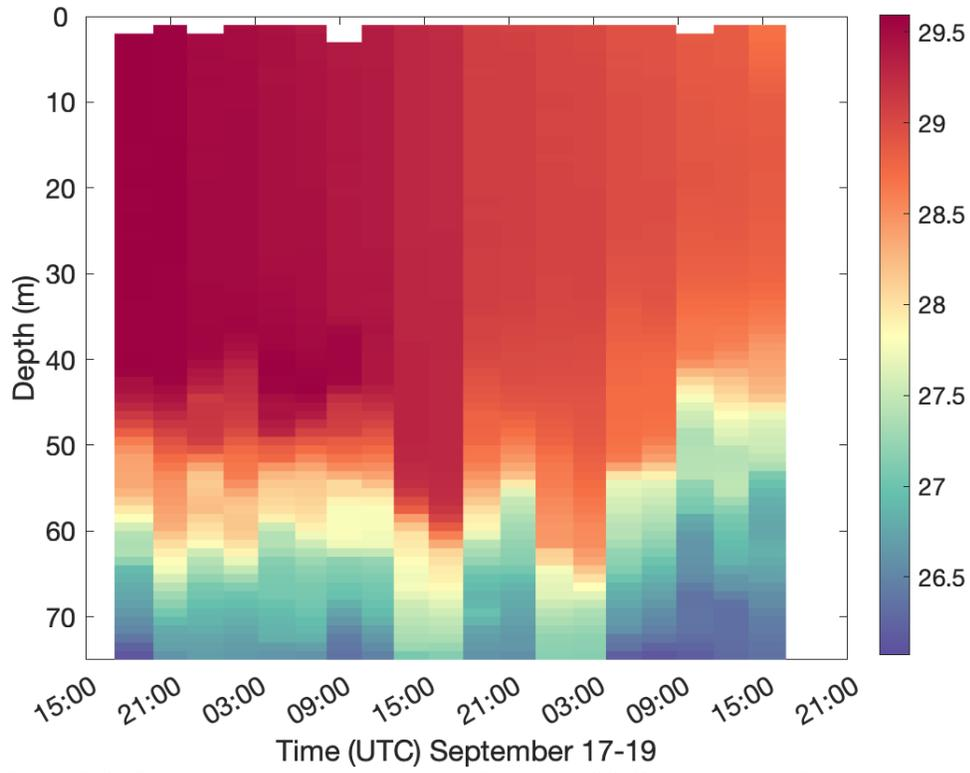
**Figure 7** Profiles of ocean temperature acquired from glider SG-610 as Hurricane Fiona passed over it.
