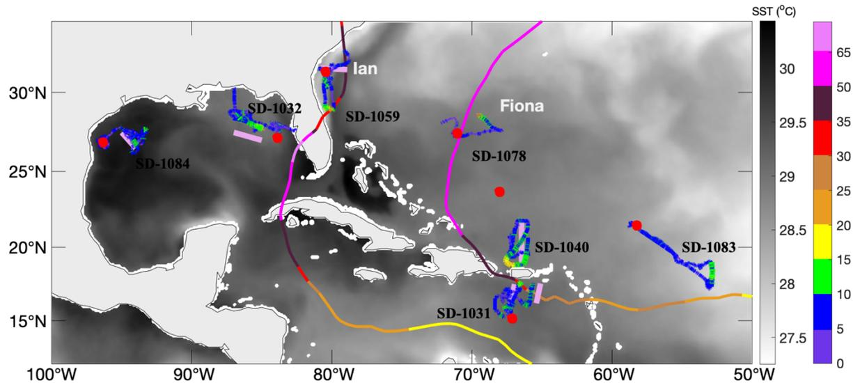
**Figure 2** Tracks of saildrones (squiggly colored lines) and their hourly-averaged wind speed measurements (color scale on the right in  $\text{m s}^{-1}$ ), underwater gliders (straight pink lines), and tropical cyclones that passed close to a saildrone (smooth lines: colors indicate maximum 1-min sustained wind speed using the color scale on the right) during the 2022 hurricane season. Red dots indicate locations of NDBC surface meteorological buoys that were compared with saildrone data.
