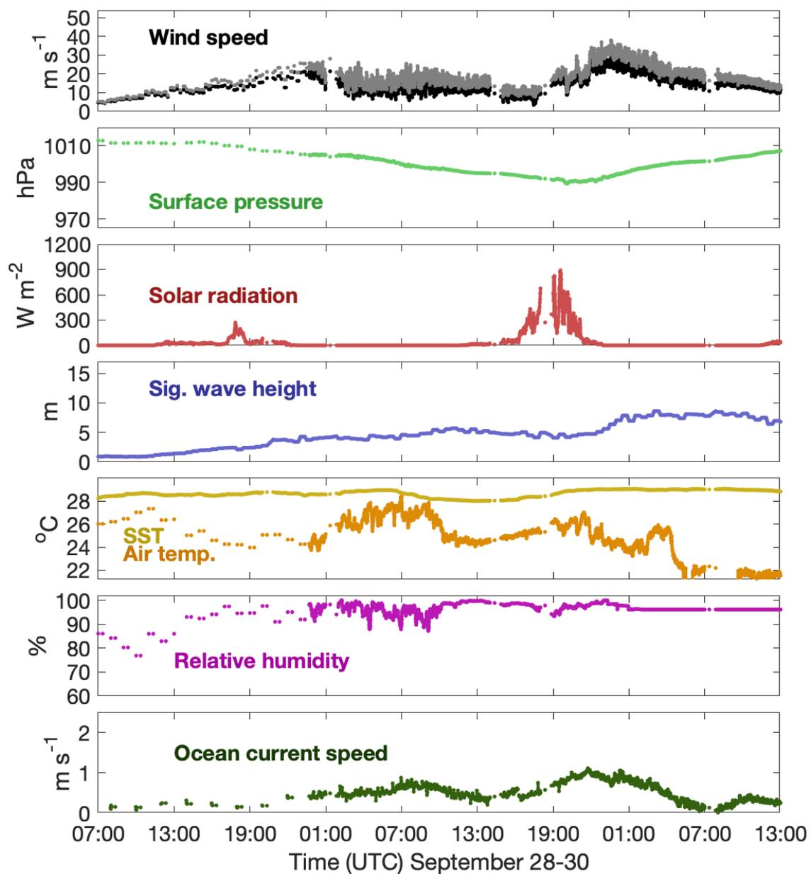
Figure 16 Key measurements (1-minute averages for most variables) from SD-1059 in Hurricane Ian.
