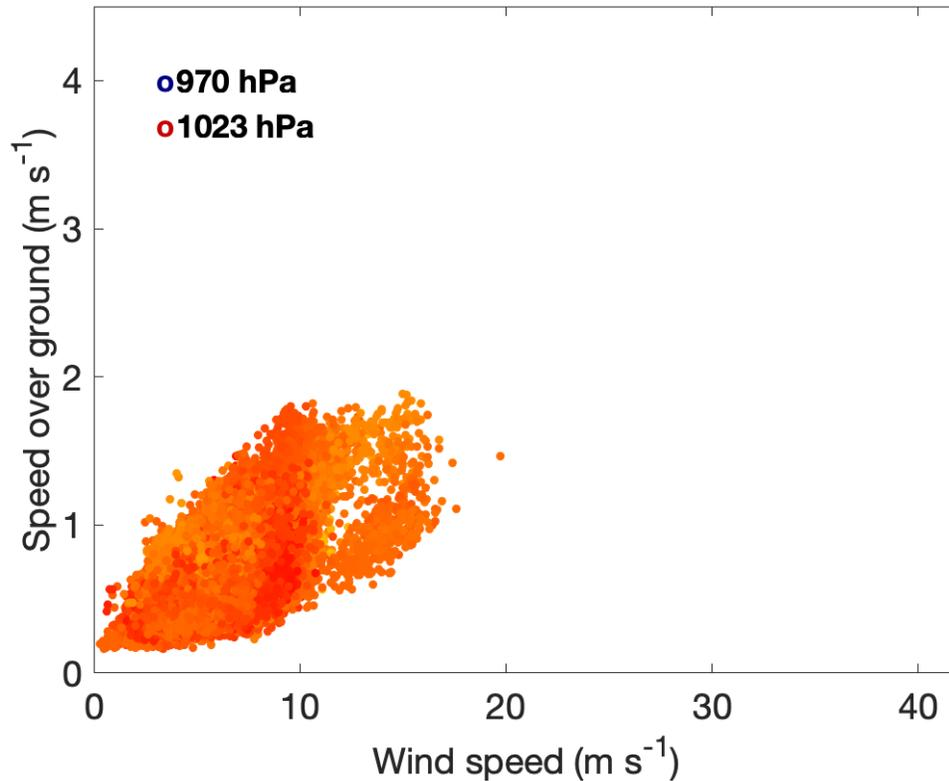
**Figure 4** Scatterplot of SD-1059's speed over ground vs. measured 1-min. wind speed for the duration of its mission, color-coded by measured barometric pressure (rainbow palette with extremes shown in legend).
