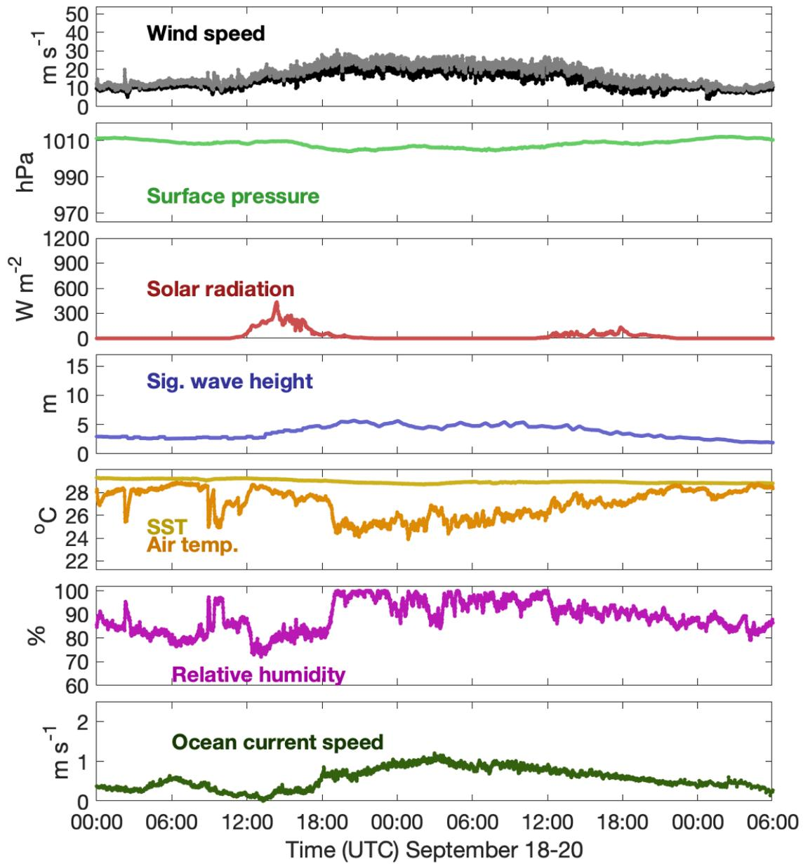
**Figure 10** Key measurements (1-minute averages for most variables) from SD-1040 in Hurricane Fiona.
