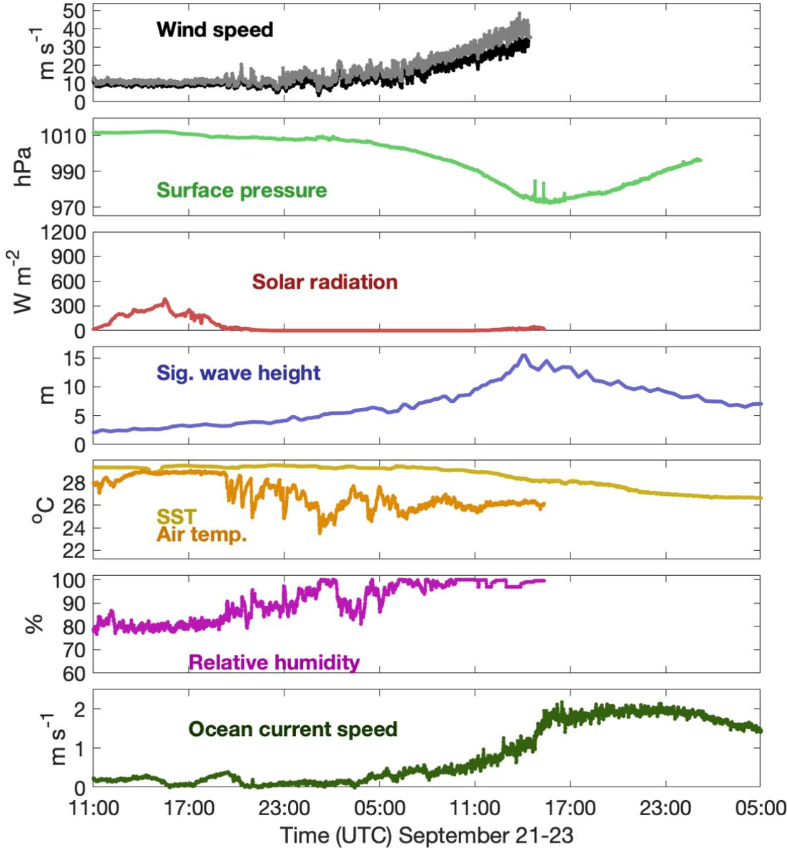
Figure 12 Key measurements (1-minute averages for most variables) from SD-1078 in Hurricane Fiona.
