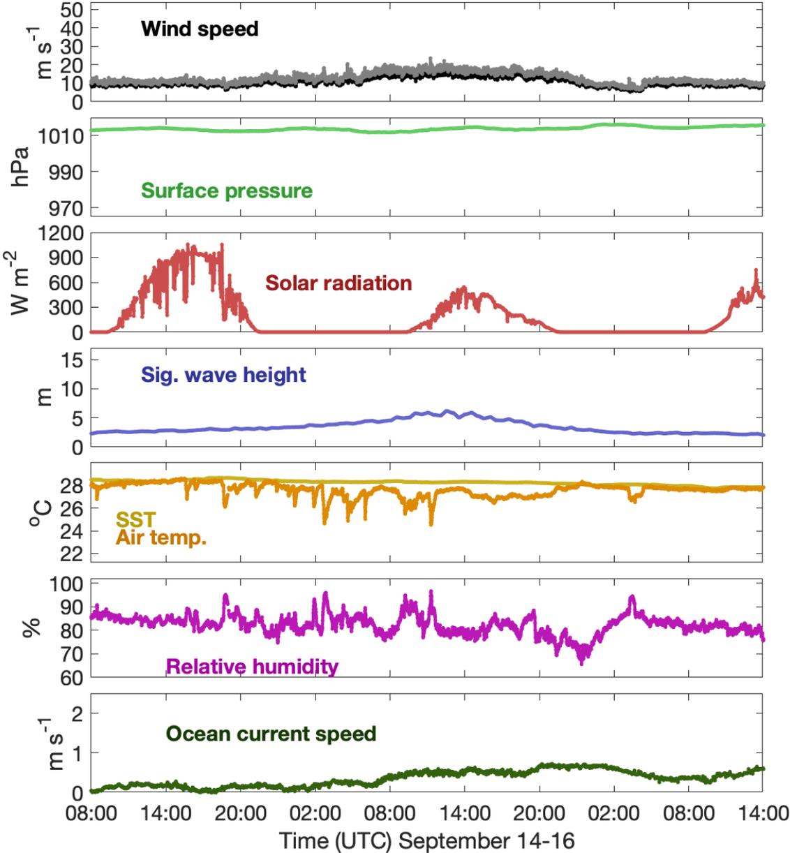
Figure 3 Key measurements (1-minute averages for most variables) from SD-1083 in Tropical Storm Fiona.
