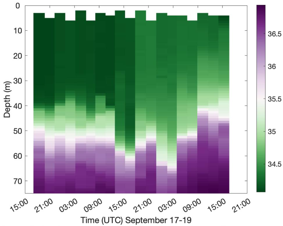
**Figure 8** Profiles of ocean salinity acquired from glider SG-610 as Hurricane Fiona passed over it.
