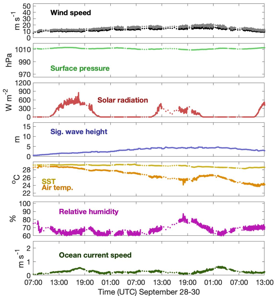
Figure 14 Key measurements (1-minute averages for most variables) from SD-1032 in Hurricane Ian.
