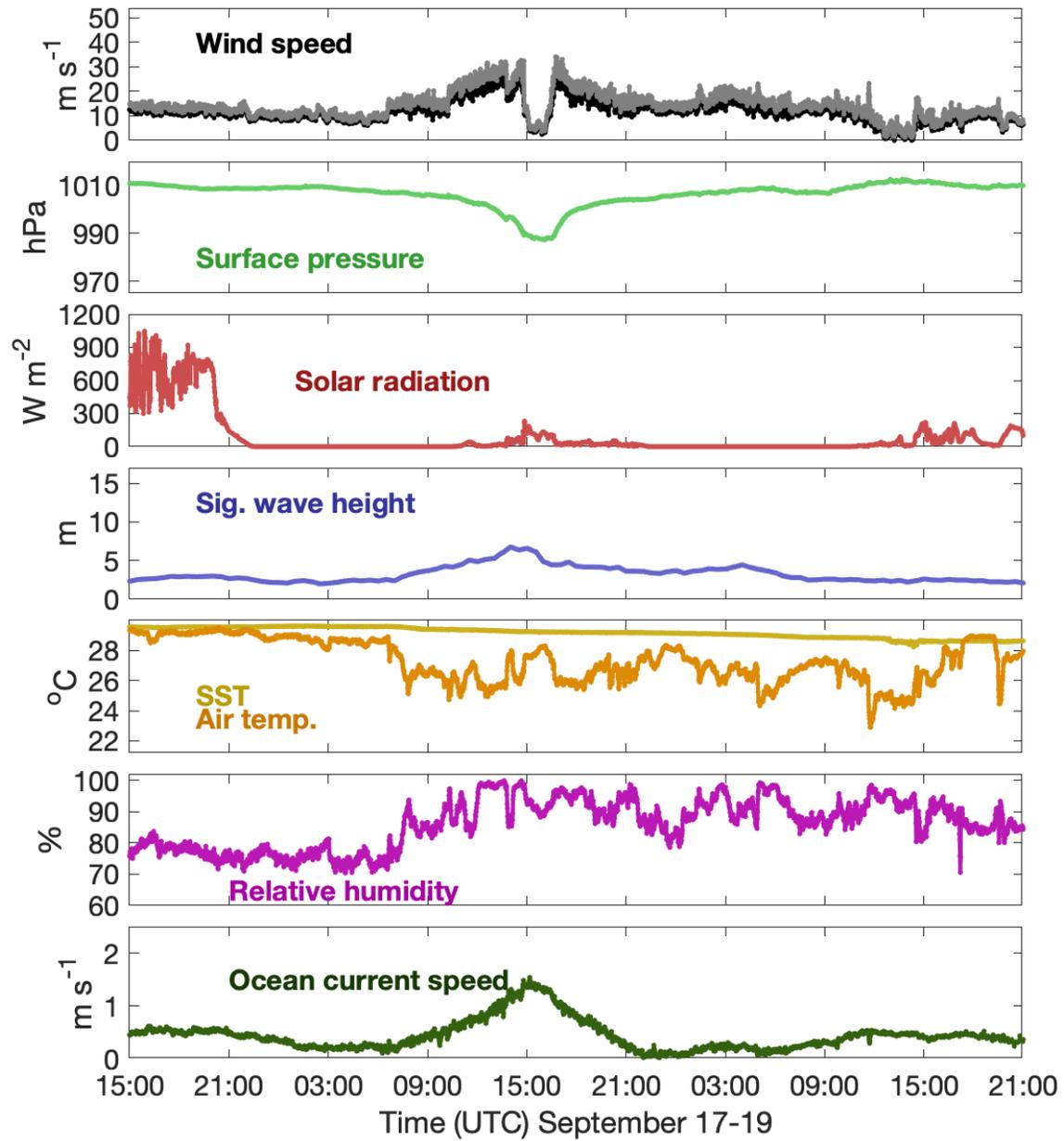
**Figure 6** Key measurements (1-minute averages for most variables) from SD-1031 in Hurricane Fiona.
