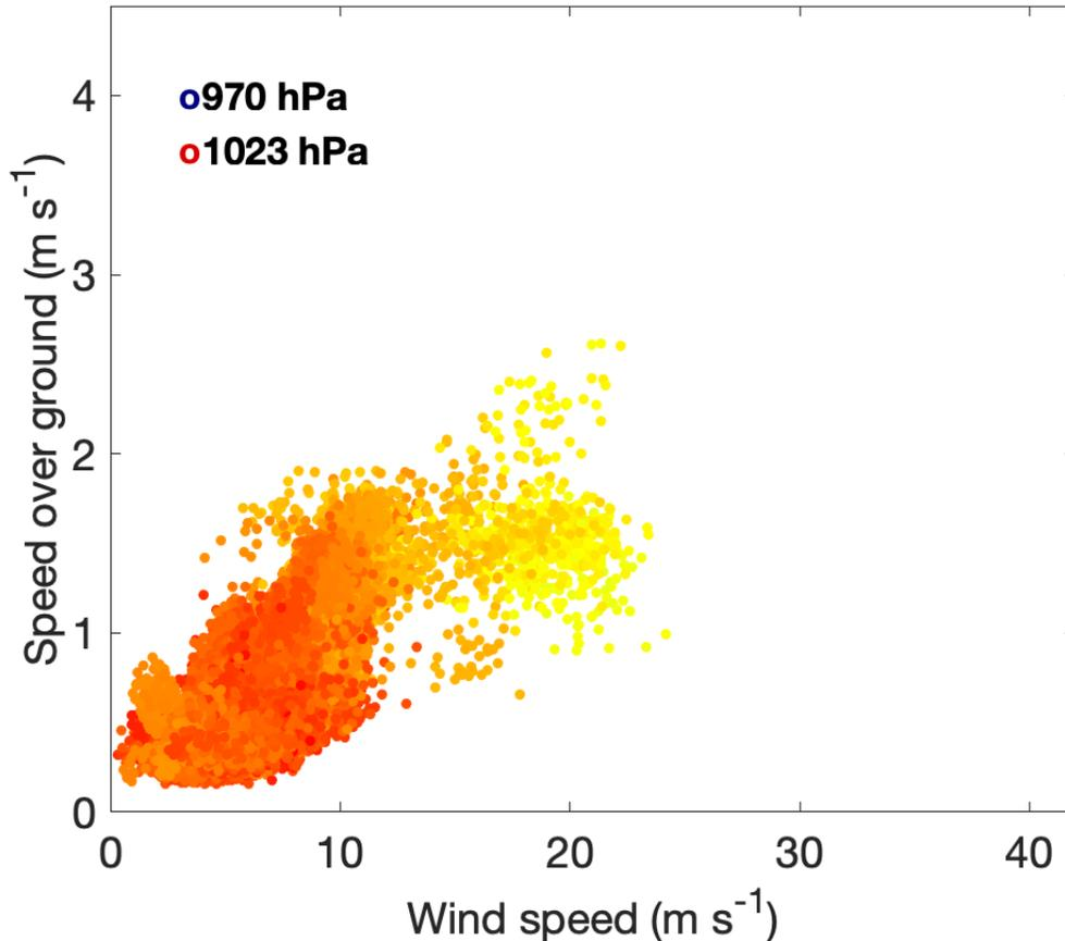
**Figure 11** Scatterplot of SD-1040's speed over ground vs. measured 1-min. wind speed for the duration of its mission, color-coded by measured barometric pressure (rainbow palette with extremes shown in legend).
