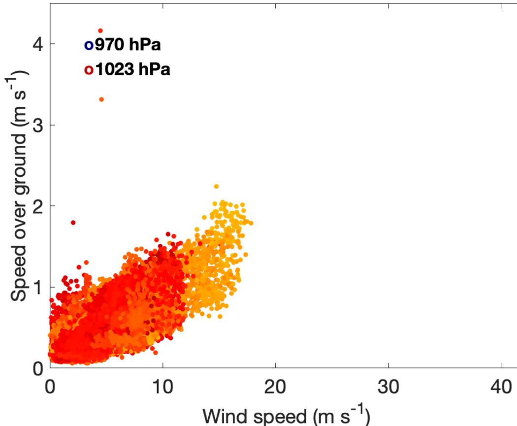
**Figure 15** Scatterplot of SD-1032's speed over ground vs. measured 1-min. wind speed for the duration of its mission, color-coded by measured barometric pressure (rainbow palette with extremes shown in legend).
