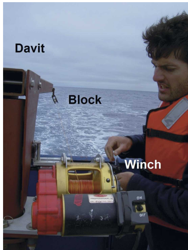
FIG. 4. UCTD winch and davit just after probe is fully deployed. The winch, davit, and block are labeled. The winch consists of a fishing reel connected through a chain (inside red case) to a motor (black housing). The davit is pointed directly aft, and the line running through the block is approaching maximum tension. The last several layers of line on the winch are colored red to remind the operator to stop paying our line.
