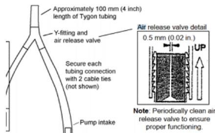
2. Blow air through the air release valve to make sure it is open.
