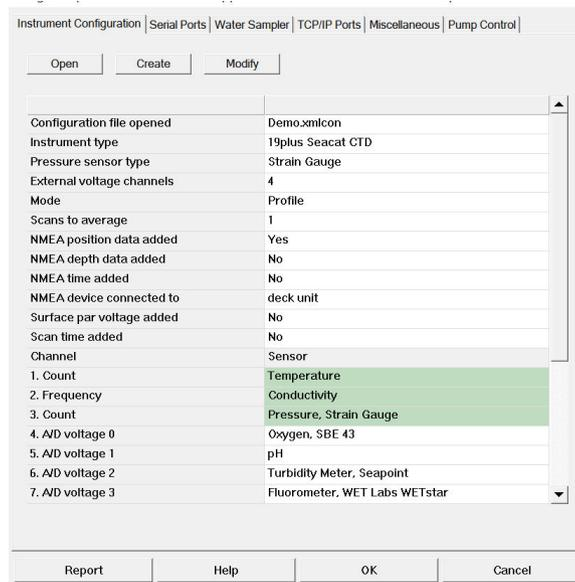
7. Make sure that the sensors are the same as the sensors attached to the 25plus, and that the channels are correct.
