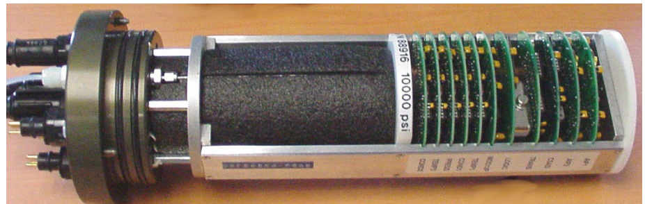
Bottom end cap PCB assembly (card file) – each PCB labeled for easy identification
