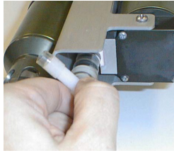
Rotate C Duct clockwise
