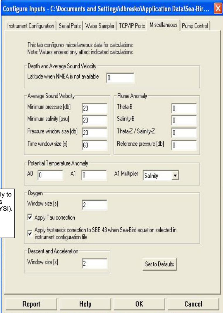
Oxygen selections apply to voltage oxygen sensors (SBE 43, or Beckman/YSI). They do not apply to SBE 63 or Aanderaa Oxygen Optode.
