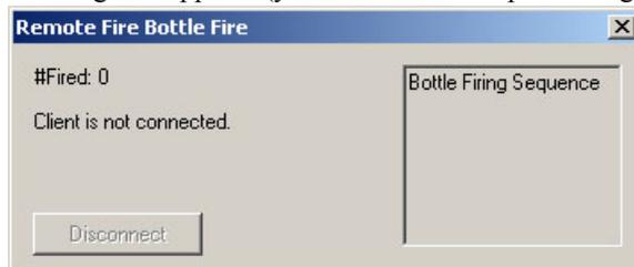
4. On the **remote computer**, double click on SeasaveRem.exe. Seasave Remote has menus, a Status bar, and fixed, scrolled, and/or plot displays, as well as a bottle fire control window.
