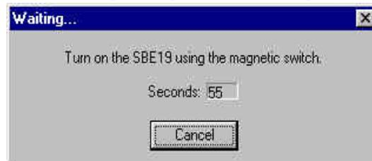
Seasave allows *Timeout in seconds at startup* after you click Start for you to turn on the CTD switch. Seasave will *time out* if data is not received from the instrument within this time.
