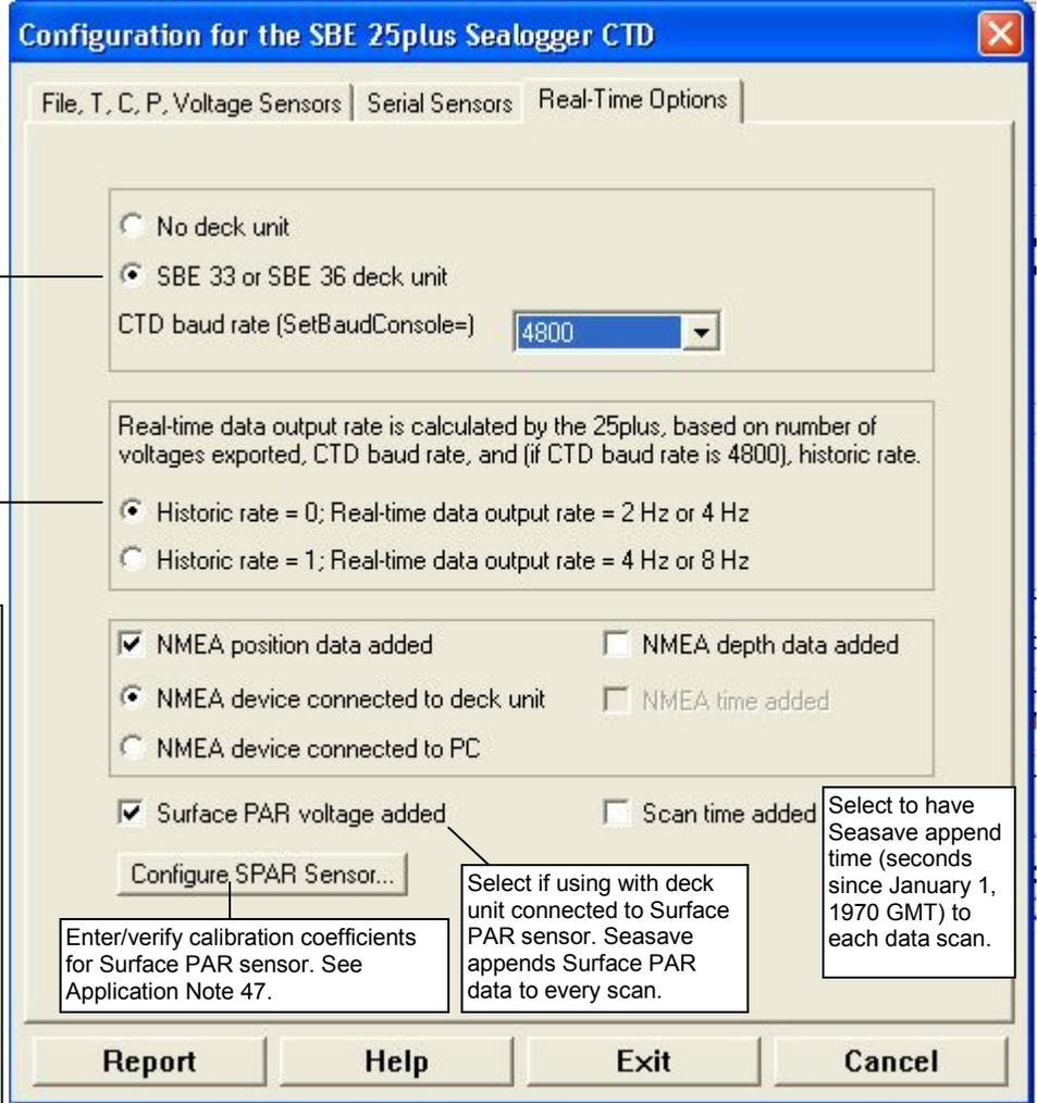
Enter/verify calibration coefficients for Surface PAR sensor. See Application Note 47.
