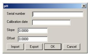
The **Export** button allows you to export coefficients for the selected sensor to an .XML file. If you move that sensor onto another instrument, you can then import the coefficients from the .XML file when setting up the .con or .xmlcon file for that instrument.
