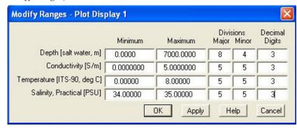
This allows you to easily and quickly modify the range for each axis. Click Apply to see how any changes look. Click OK to exit the dialog box; all changes will be retained (but you can undo the changes if desired, using the Undo button on the plot toolbar).
