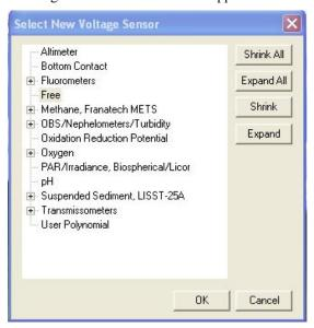
Double click on the desired sensor. The Calibration Coefficients dialog box appears. An example is shown below for a pH sensor:
