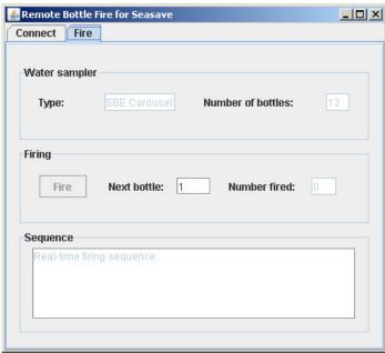
If the remote software is working properly, the water sampler type and number of bottles should match the settings on the Water Sampler tab in Configure Inputs in Seasave.
