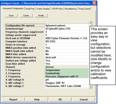
Click Modify to bring up a dialog box to change the configuration and/or view calibration coefficients.
