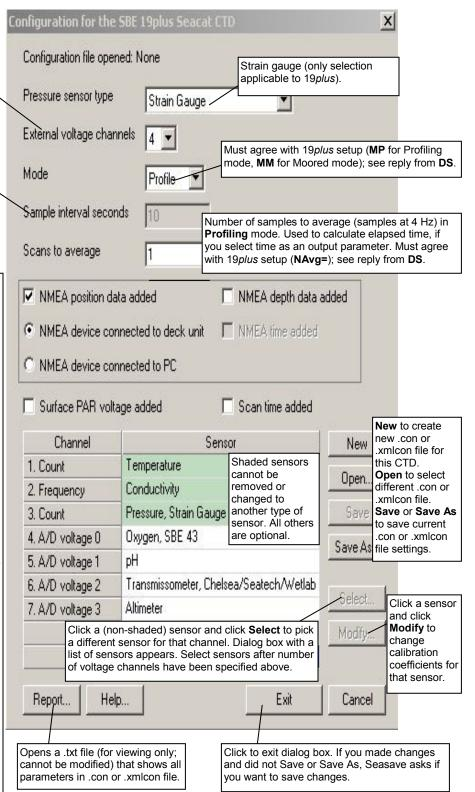
Shown below is an example status (**DS**) response *in Seaterm* that corresponds to the setup shown in the Configuration dialog box above. Shown below the appropriate lines are the commands used in Seaterm to modify the setup of parameters critical to use of the instrument with Seasave, as well as any explanatory information.
