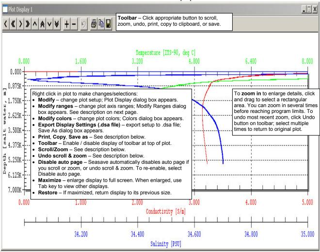
Change the plot using the toolbar buttons **or** by right clicking in the plot:
