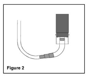
This application note provides instructions for use of PN 50087 / 50087.1 syringe and tubing assembly in rinsing, cleaning, and storing conductivity sensors. The tubing assembly consists of a length of 6.35 mm (1/4 inch) I.D. tube connected by a plastic reducing union to a short piece of 11.1 mm (7/16 inch) I.D. tube. Refer to *Application Note 2D: Instructions for Care and Cleaning of Conductivity Cells* for information on water and solutions recommended for use.
