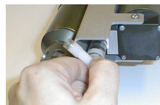
Temperature sensor guard rotated 90° counterclockwise while C Duct rotated clockwise slightly
