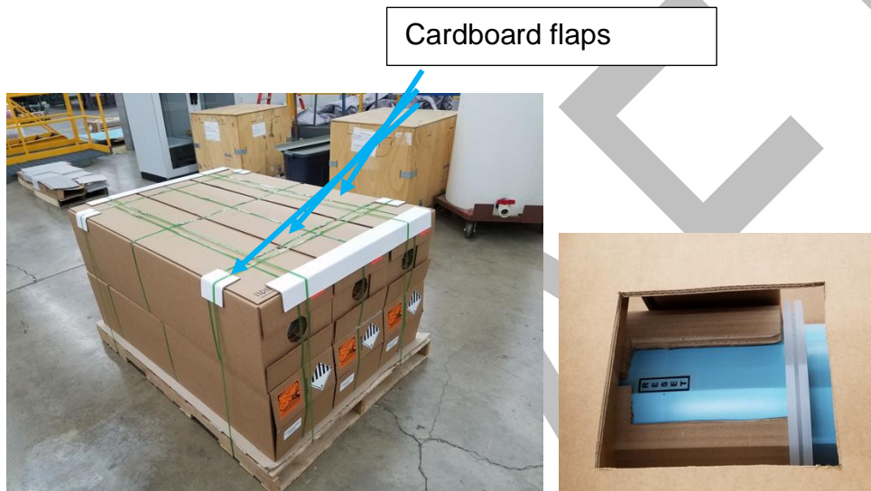
Figure 8a and 8b. ALTO with parachute ready for aircraft aft cargo-door launch. Note location of the access window for the RESET label (Figure 8b).
