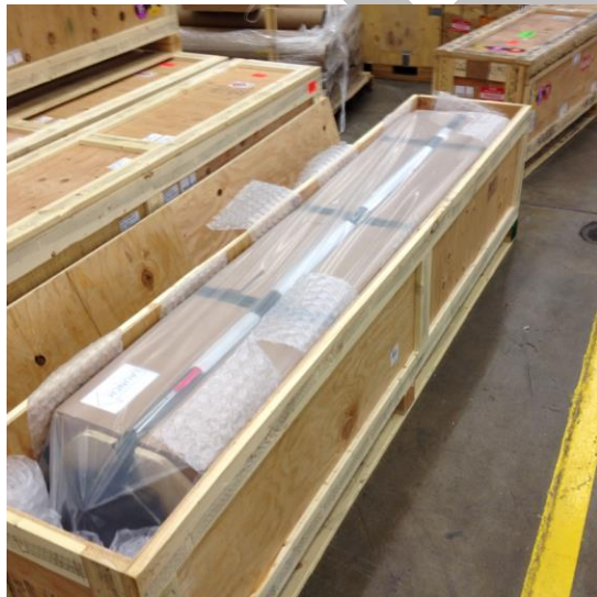
Figure 9c ALTO in protective bag with harness in shipping crate showing parachute end.
