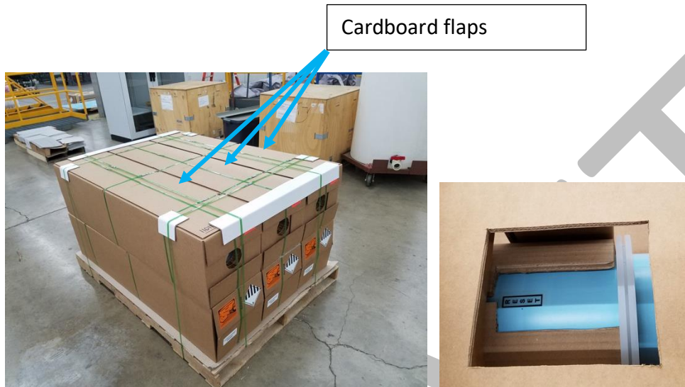
Figure 9a and 9b. ALTO with parachute ready for aircraft aft cargo-door launch. THIS IS NOT CORRECT. THIS IS A PALLET OF SIX ALTOS READY FOR SHIPMENT. IT SHOWS THE LOCATION OF THE CARDBOARD FLAPS THAT AFFORD ACCESS TO THE RESET LABEL... Note location of the access window for the RESET label (Figure 9b).
