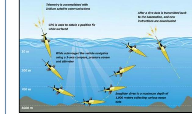
changes in buoyancy together with wings to propel itself by converting vertical motion into horizontal motion. Thanks to a very small consumption of energy, underwater gliders have longer ranges when compared to other AUVs, being able to measure several ocean parameters during months, including temperature, salinity, and dissolved oxygen.
