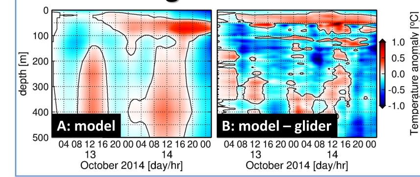
The model overestimated the surface cooling by 0.2°C, possibly because of discrepancies in initial conditions for salinity. Larger SST cooling in the model may have lead to an underestimated intensity forecast for Gonzalo.
