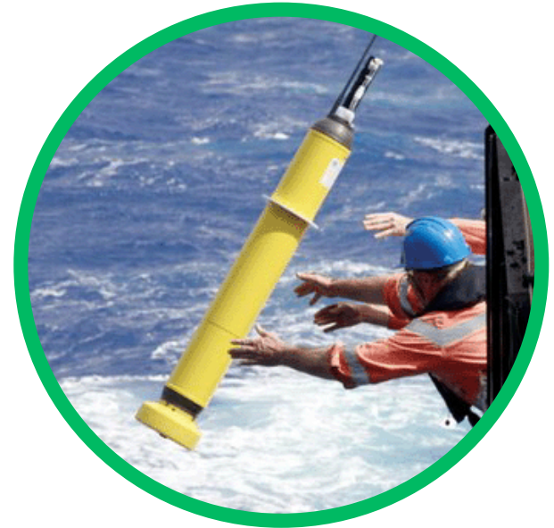
Argo float ( autonomous CTD "robot" )
