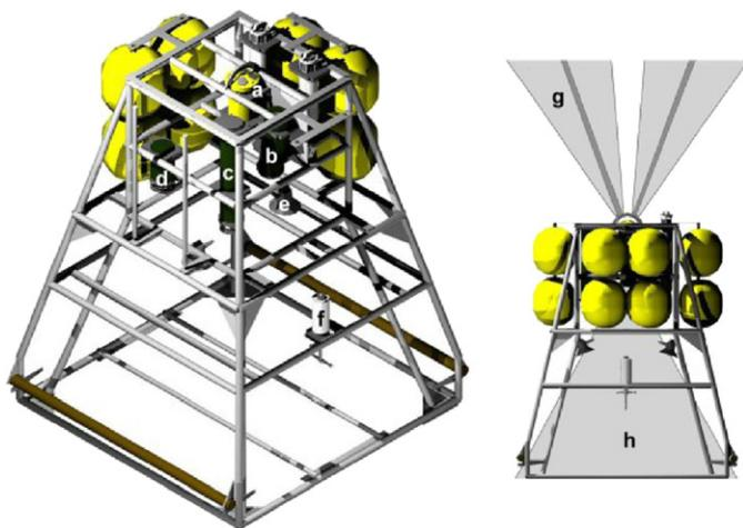
Fig. 7. The DOBO lander. The DOBO is equipped with an acoustic Doppler current profiler (ADCP) (a), 35 mm stills camera in time-lapse mode (capacity 1400 frames) (b), battery (c), controller (d), flash system (e), FSI current meter (f), and bait system (not shown). The upward-looking ADCP records current velocity and direction in 3-m depth cells above the lander (g). The camera photographs the bait system arranged at the base of the lander (h). Source: OCEANLAB, University of Aberdeen.
