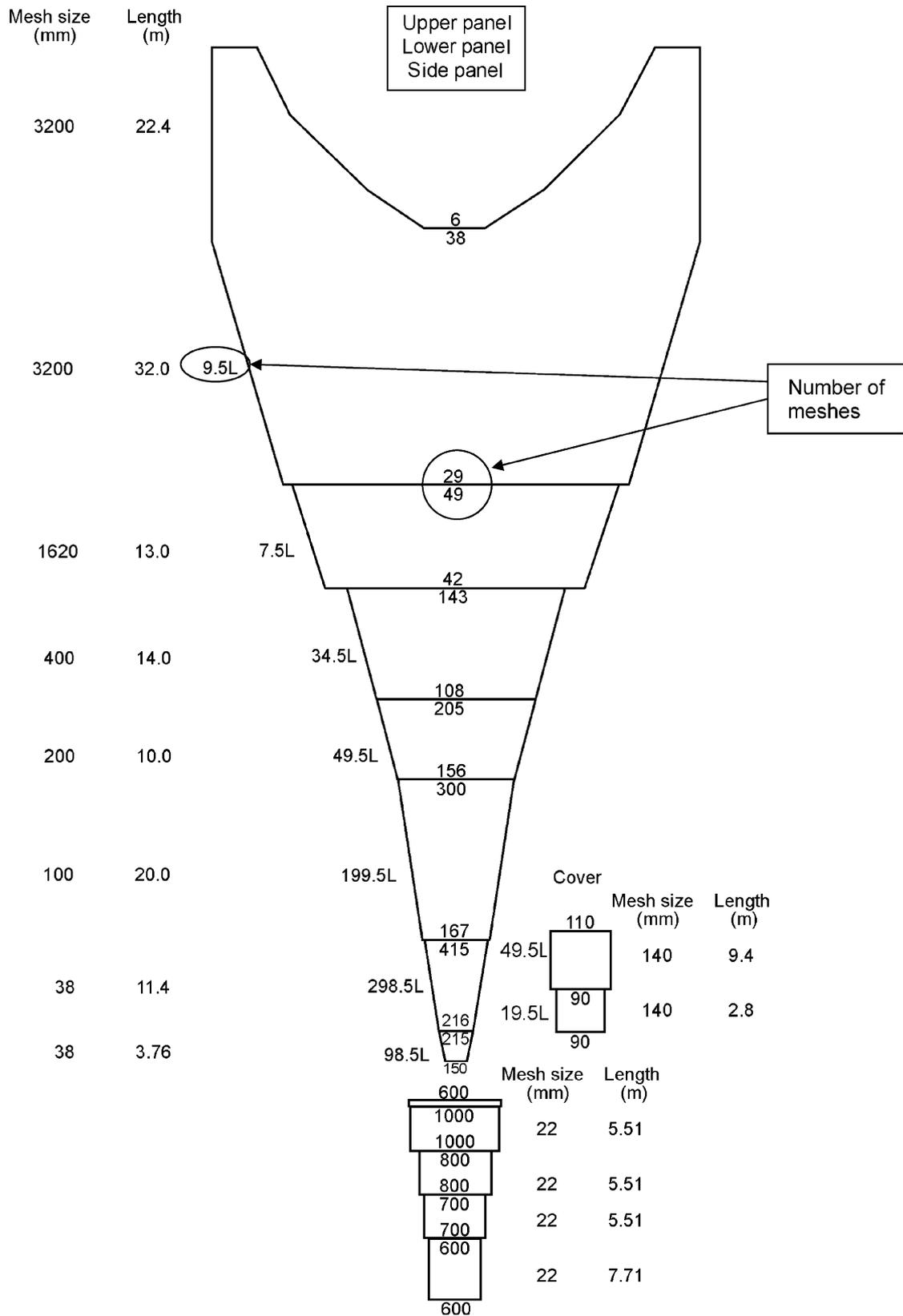
Fig. 3. Manufacturer's diagram of the "Aakratrawl", the medium-sized pelagic fish trawl used routinely for depth-stratified sampling during Leg 1 of the 2004 MAR-ECO expedition. The diagram shows dimensions and stretched mesh sizes and numbers for one of the four equal net panels that the trawl consists of, plus the codend and protective cover. Three equal codends were used and these were attached to a multisampler that facilitated opening and closing during the tow.
