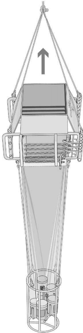
Fig. 4. Sketch of the Multinet used for depth-stratified sampling of mesozooplankton during the 2004 MAR-ECO expedition. Source: HYDRO-BIOS Apparatebau GmbH.
