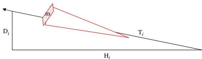
Fig. 6. Calculation of volume filtered water by the macrozooplankton trawl:  $T_i$  = towing distance at depth interval  $i$ ,  $m$  = area of the mouth opening of the trawl (36m<sup>2</sup>),  $D_i$  = height of the depth interval  $i$ , and  $H_i$  = horizontal distance covered while trawling at depth interval  $i$ .
