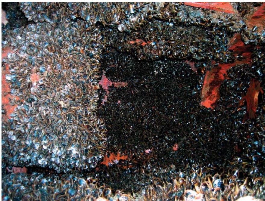
Figure 2. Fouling assemblages in the sea-chests of the SA Agulhas were dominated by Mytilus galloprovincialis
