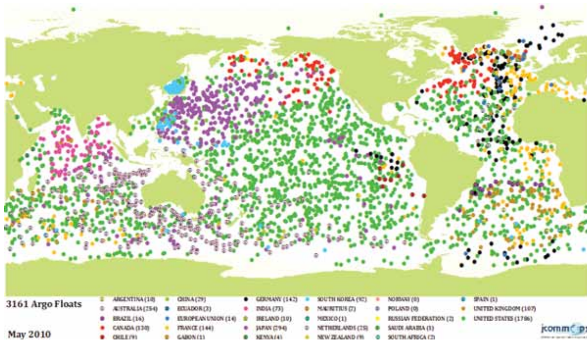
Figure 5. Distribution of Argo floats (as of May 31, 2010) in the world's ocean. Today, over 3000 Argo floats have been released (given an average lifetime of 3.75 years, approximately 800 floats must be released each year to sustain the desired standing stock of 3000 active floats). Source: http://wo.jcommops.org/cgi-bin/WebObjects/Argo.woa/1/wo
