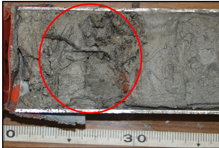
Red circle indicates area sampled for GC/MS.
