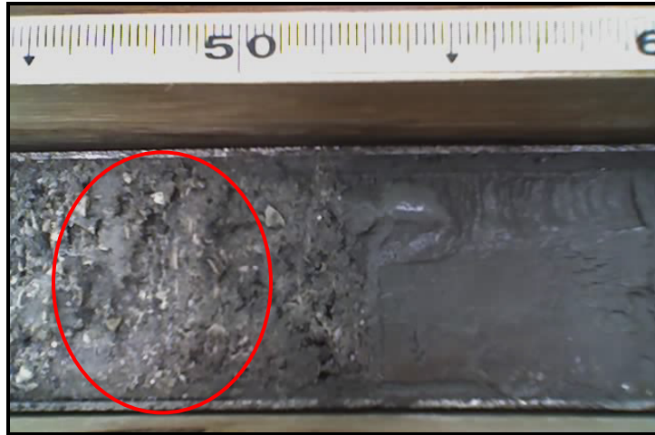
Red circle indicates area sampled for GC/MS.
