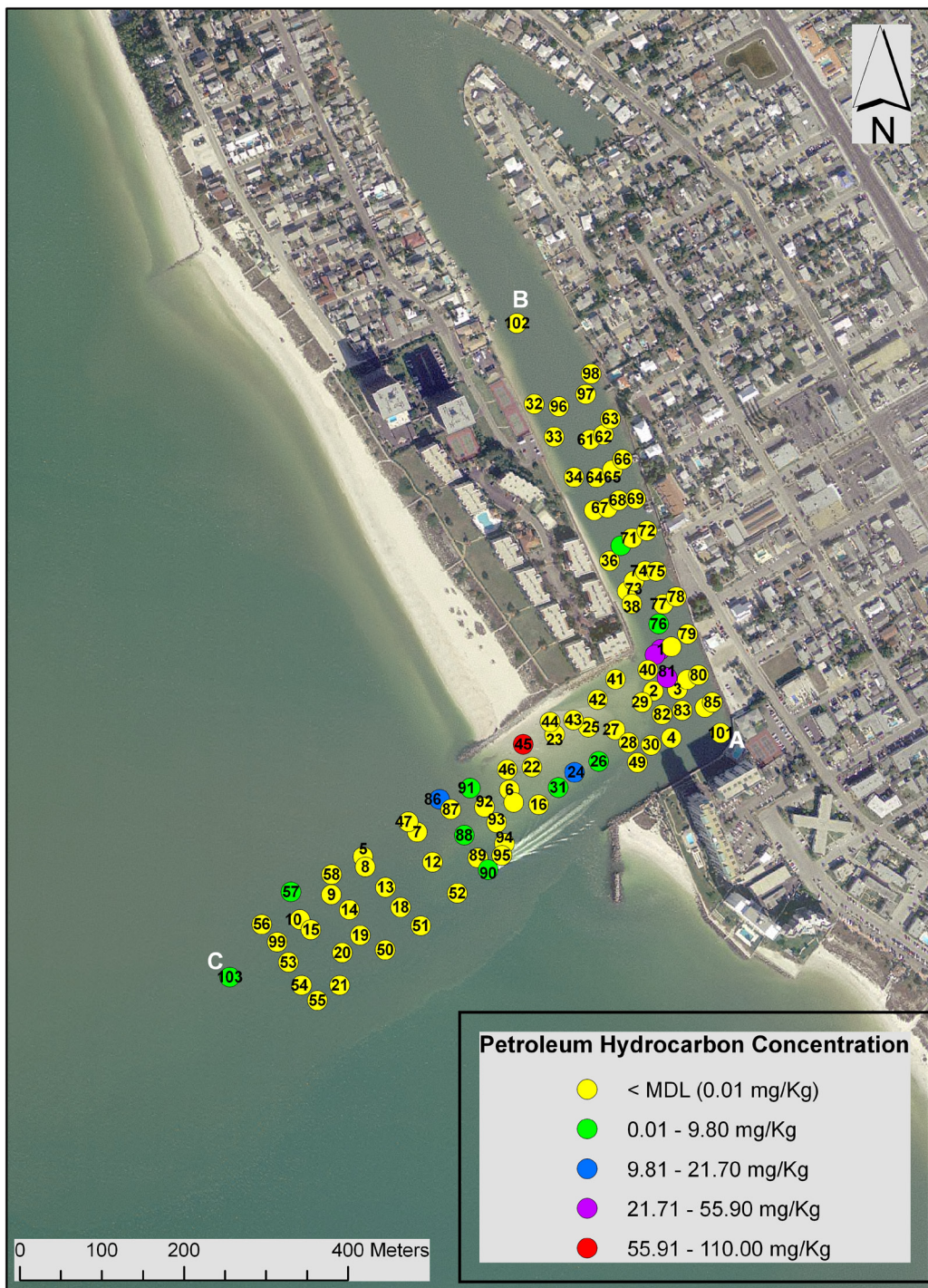
Figure 32: Spatial distribution of total petroleum hydrocarbons at the 200-299 cm depth interval in Blind Pass.
