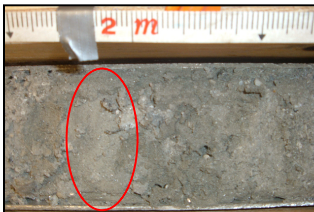
Red circle indicates area sampled for GC/MS.
