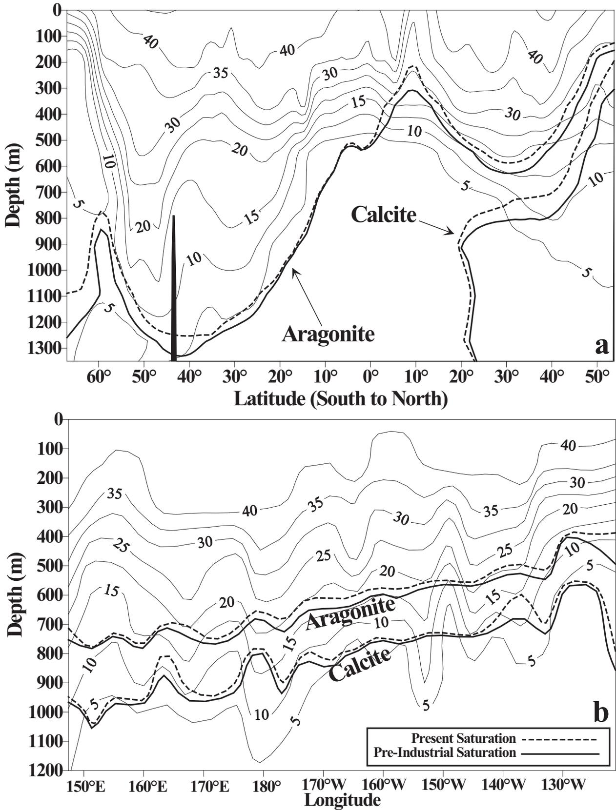
**Figure 6.** Vertical distributions of anthropogenic CO<sub>2</sub> concentrations in  $\mu\text{mol kg}^{-1}$  and the supersaturation/undersaturation horizons for aragonite and calcite along (a) WOCE/JGOFS section P15S and P15N, and (b) WOCE/JGOFS section P2 in the Pacific Ocean.
