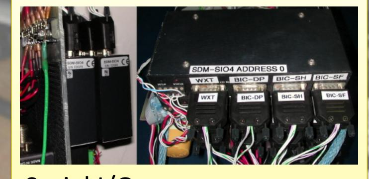
Serial I/O (Campbell Scientific SDM-SIO4) Instruments which communicate via serial RS-232 connections plug into a port on one of two 4-port interfaces which in turn connect to the datalogger. Future control units may expand to include three such units (12 serial connections, total).
