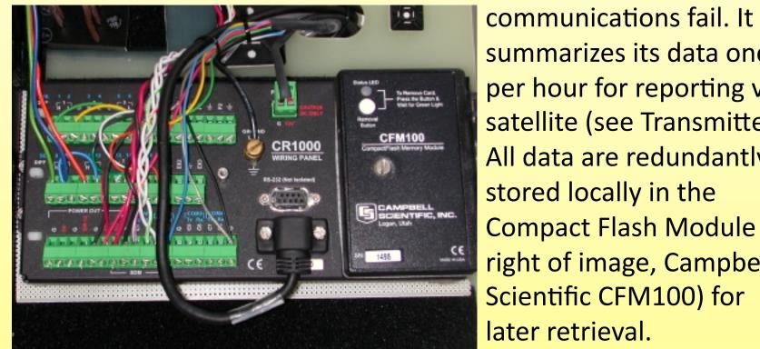
summarizes its data once per hour for reporting via satellite (see Transmitter). All data are redundantly stored locally in the Compact Flash Module (at right of image, Campbell Scientific CFM100) for later retrieval.
