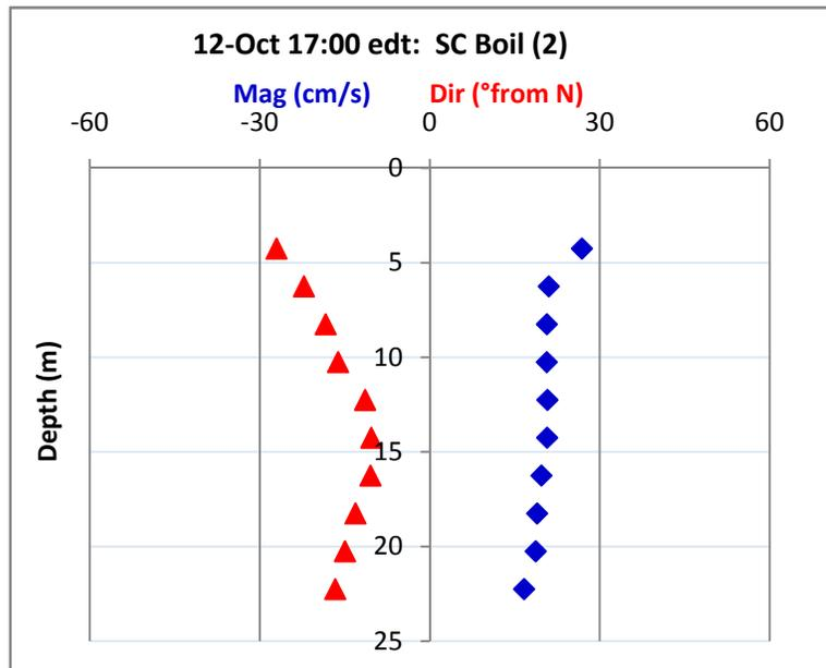
**Figure 86:** Current velocity and direction for South Central outfall on October 12, 2006 at 17:00.
