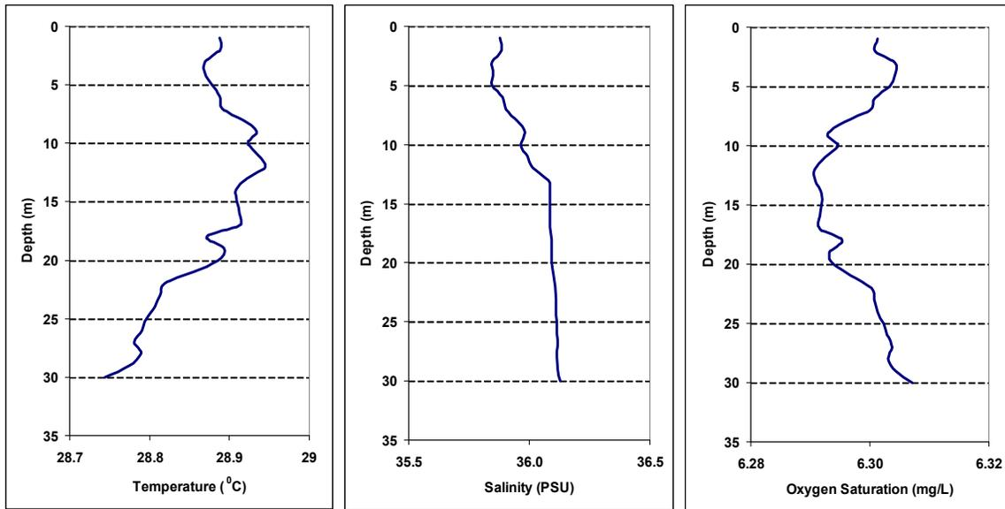
Figure 54: October 14th, 2006 temperature, salinity and oxygen concentration profile at station BRB-2.
