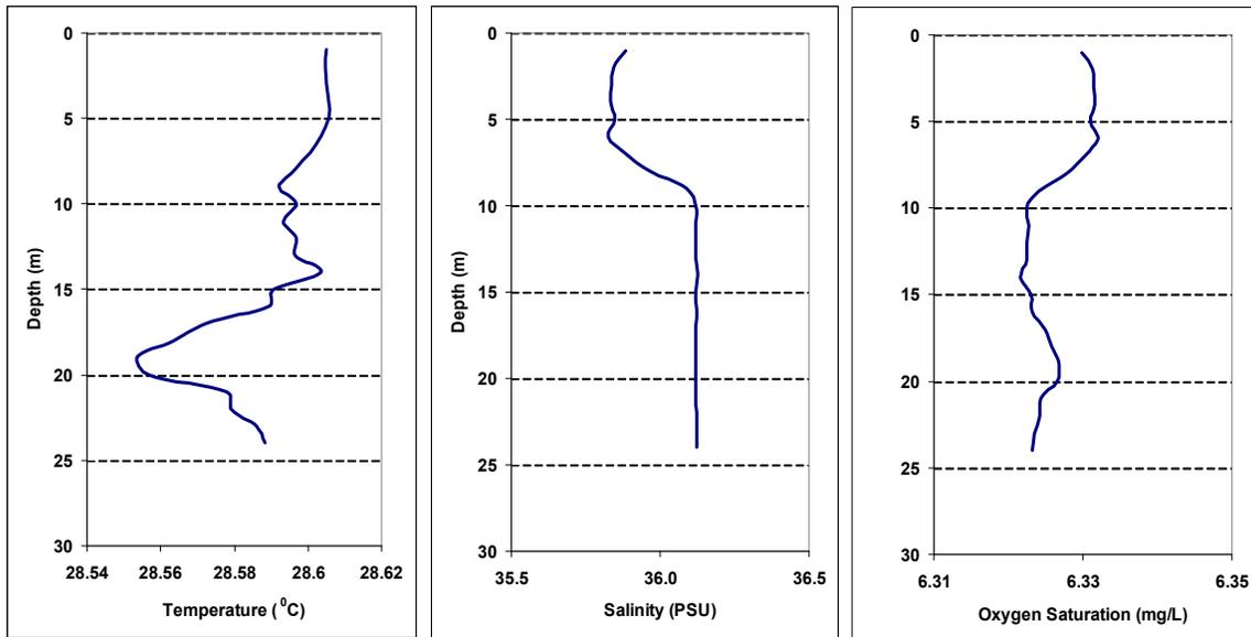
Figure 11: October 16<sup>th</sup>, 2006 temperature, salinity and oxygen concentration profile at station MCB-7.
