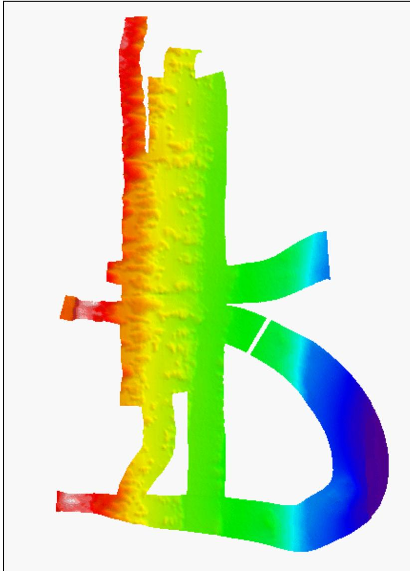
**Figure 69. Multibeam data from the vicinity of the Hollywood outfall. Structure is the small horizontal line near the center of the view.**
