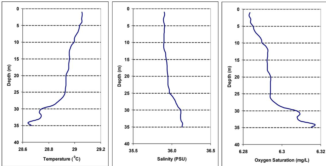
Figure 62: October 14th, 2006 temperature, salinity and oxygen concentration profile at station BRB-10.
