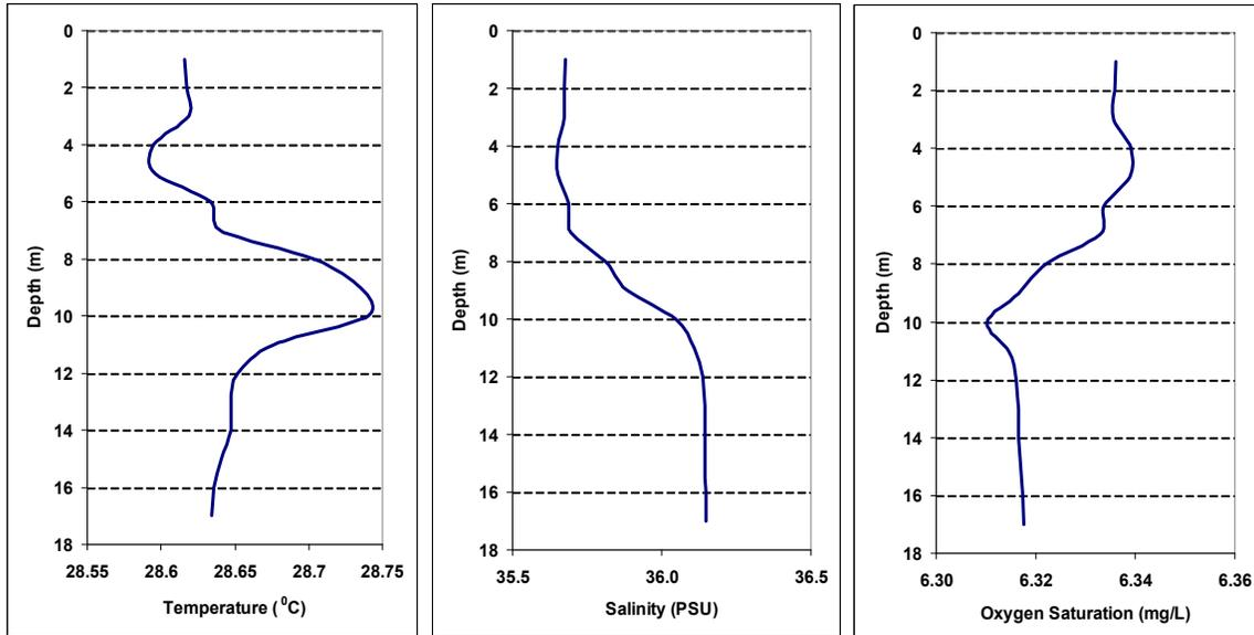
Figure 28: October 18<sup>th</sup>, 2006 temperature, salinity and oxygen concentration profile at station MNB-9.
