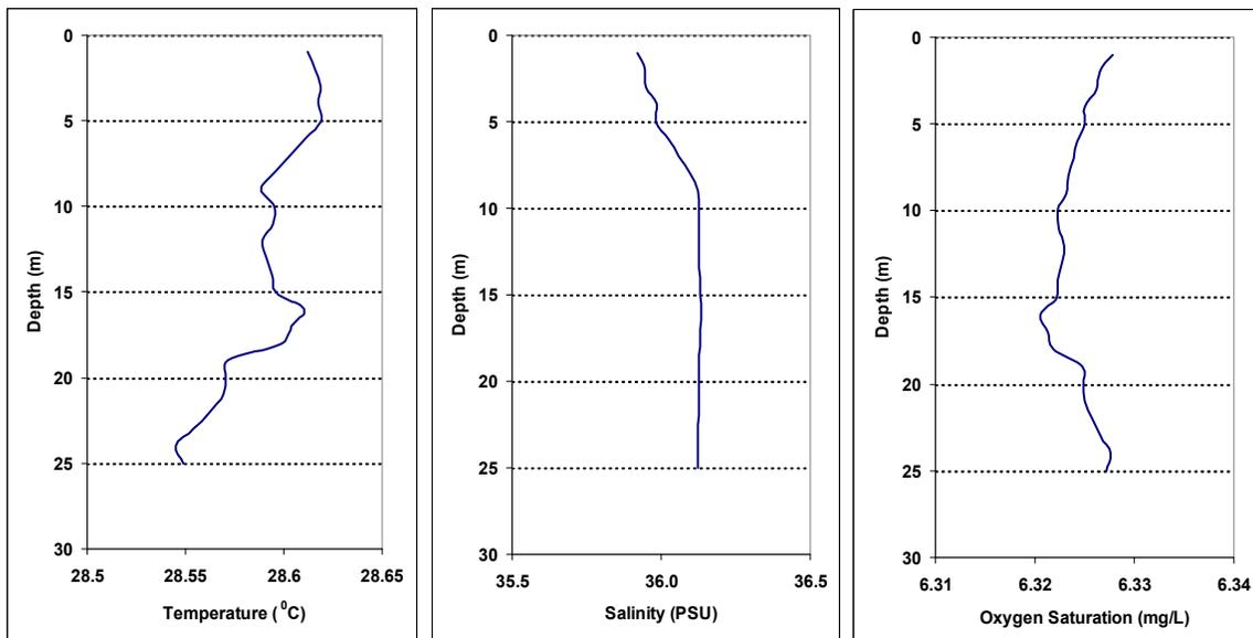
Figure 13: October 16<sup>th</sup>, 2006 temperature, salinity and oxygen concentration profile at station MCB-9.
