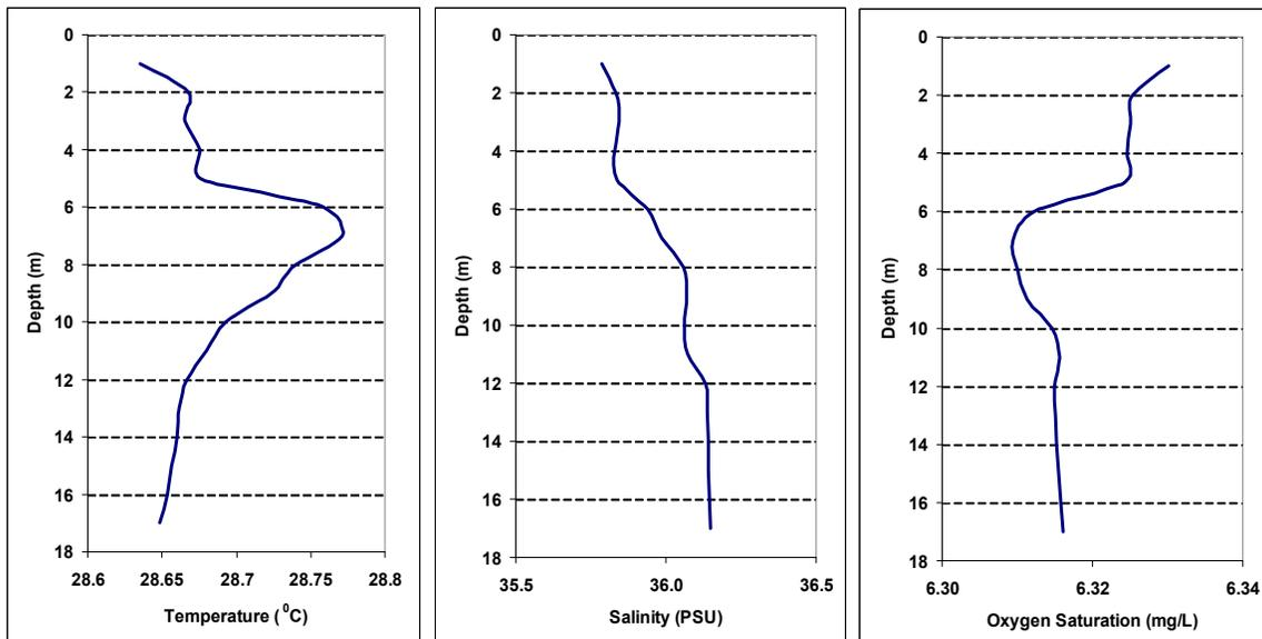
**Figure 29: October 18<sup>th</sup>, 2006 temperature, salinity and oxygen concentration profile at station MNB-10.**
