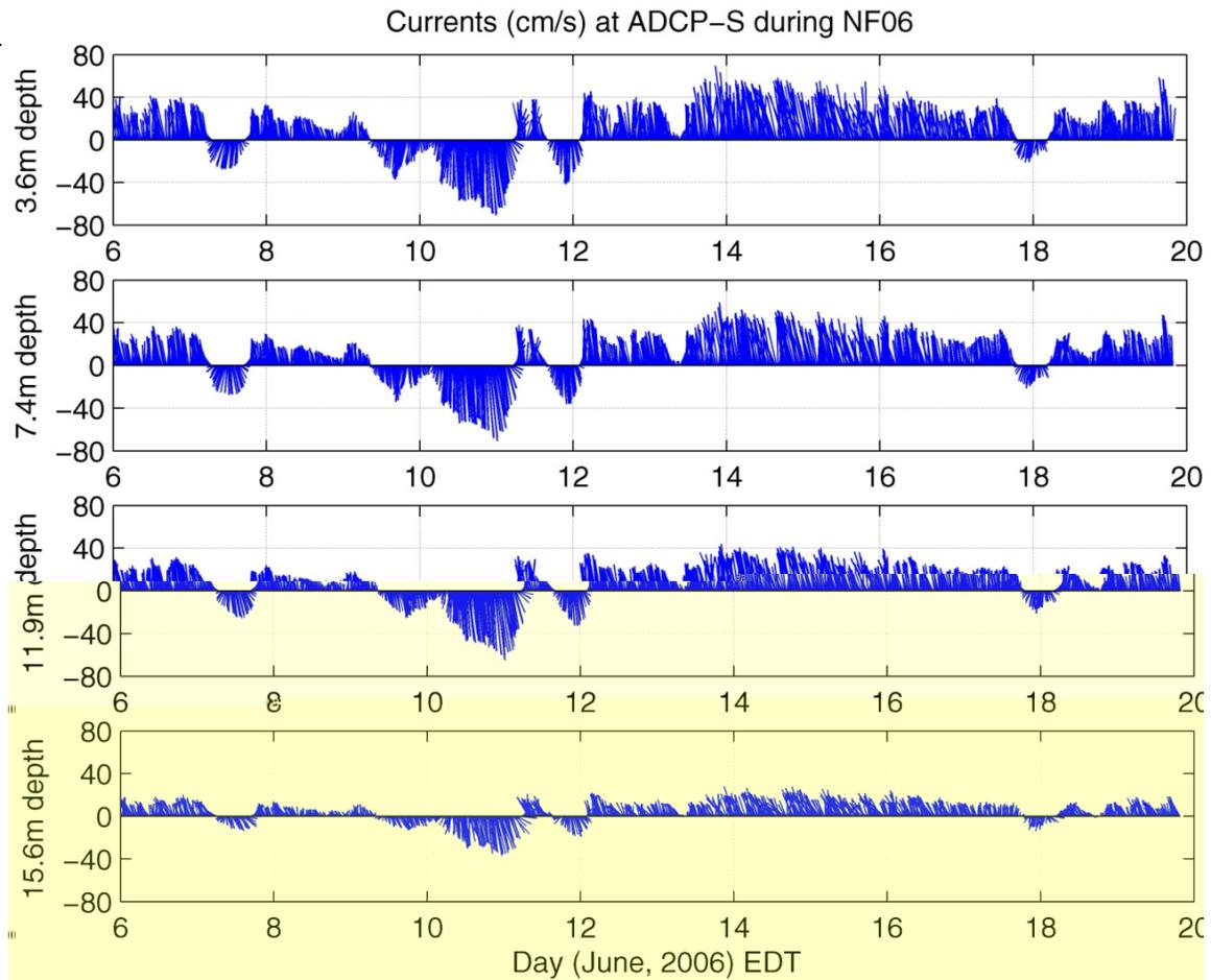
**Figure 103:** Stick plots of current data from the GSR-S ADCP instruments at depths near the surface (upper panel) to lower depths (lower panels). As with GSRN, the current at GSR-S was northerly.
