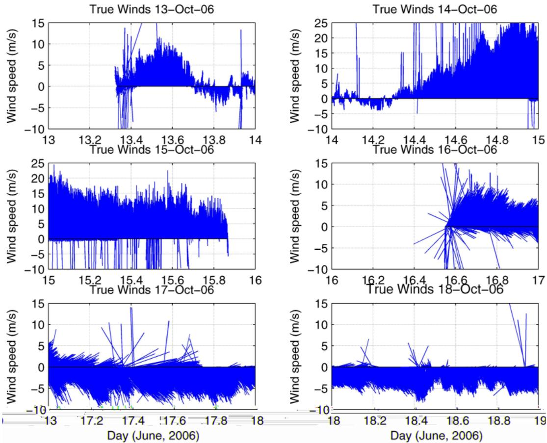
**Figure 105: Ship's true wind speed as wind barbs. This data is obtained by correcting mast wind speed and direction for ship's orientation and motion.**
