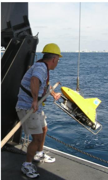
Figure 16: V-Fin being launched from the aft of the R/V Nancy Foster.
