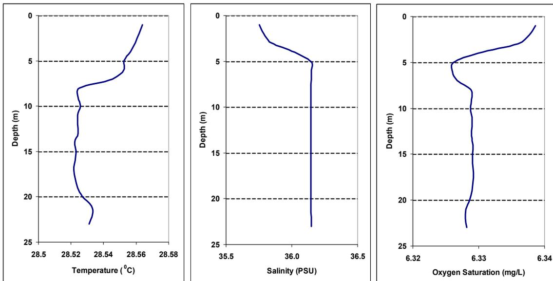
Figure 25: October 18<sup>th</sup>, 2006 temperature, salinity and oxygen concentration profile at station MNB-6.
