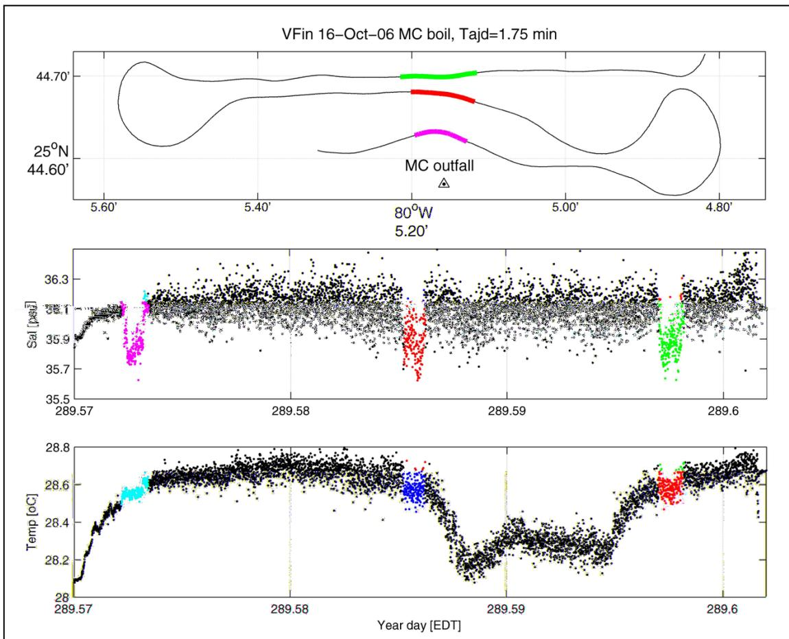
**Figure 17: Upper panel: plot of the path of the V-Fin on 16-October, crossing the Miami Central outfall plume. The middle panel (salinity) and the bottom panel (temperature) are from the V-Fin CTD instrumentation. Plume indications as determined by salinity deficit are highlighted in magenta, red, and green.**
