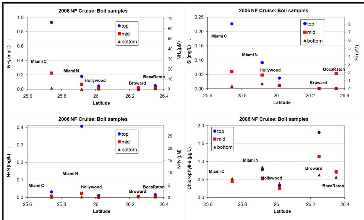
Figure 106: Nutrient results from boil samples from the five outfalls (results are not available for South Central) for  $\text{NH}_4$  (top left), N+N (bottom left), and Si (to right, plotted versus the latitude of the outfall). Units are given as mg/L (left vertical axis) and in  $\mu\text{M}$  (right vertical axis). Bottom right panel shows chlorophyll-a results ( $\mu\text{g/L}$ ).
