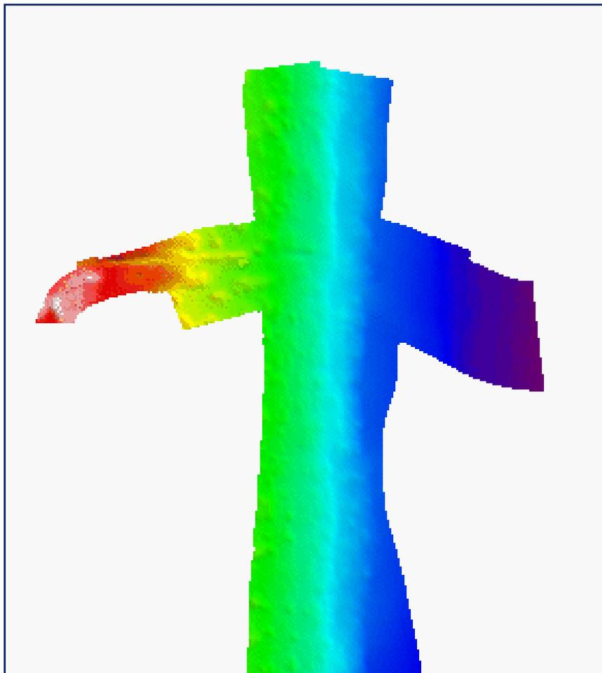
**Figure 35. Multibeam view of the sea floor in the vicinity of the Hollywood outfall pipe. The structure can be seen as the yellow line in the left arm of the view.**
