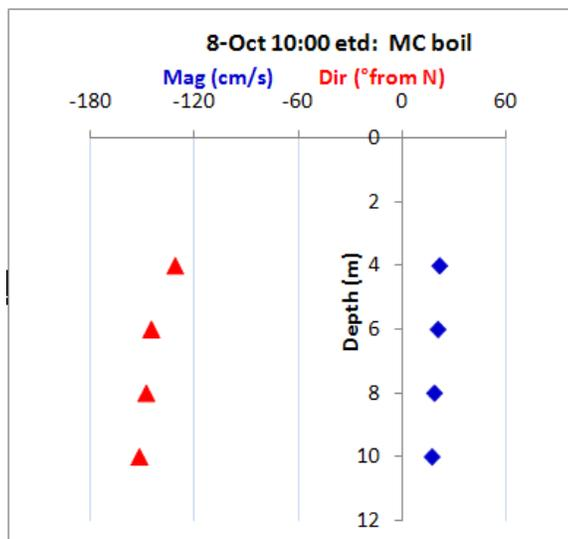
Figure 15: Current velocity and direction for Miami Central outfall on October 8, 2006 at 10:00.
