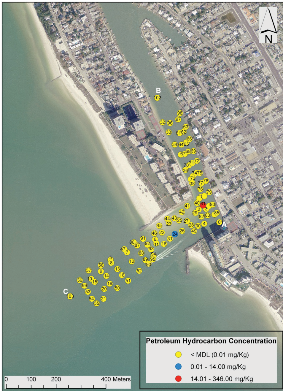
Figure 33: Spatial distribution of total petroleum hydrocarbons at the 300-399 cm depth interval in Blind Pass.
