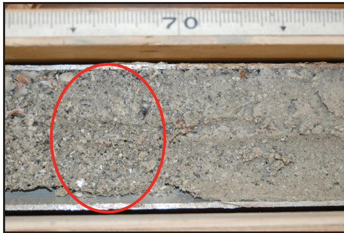
Figure 6: Subsample of sediment core JP-6 (65-70 cm).
