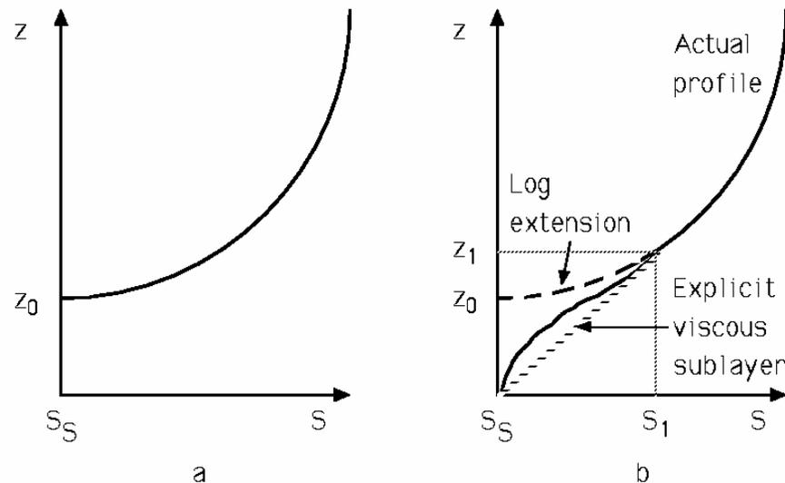
Fig. 1. Log profile ending (a), and log profile with viscous sublayer ending (b).
