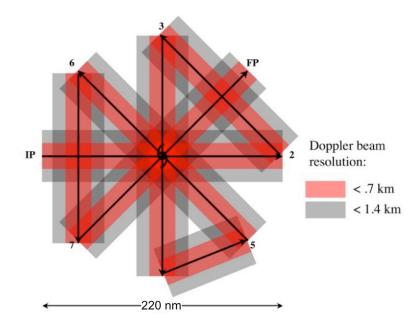
Fig. 2. Sample P-3 rotated figure-4 flight pattern. The red shading denotes locations where vertical spacing of Doppler beam < 0.7 km, grey shading where vertical spacing < 1.4 km. GPS dropsondes should be released at all turn points (past the turn after the aircraft has leveled), at midpoints of inbound/outbound legs, at the centers point between IP/2 and 5/6, and across the TC diurnal pulse.
