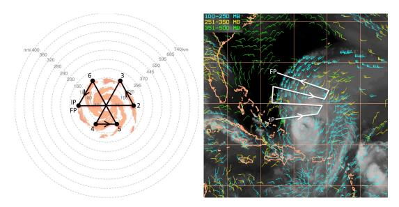
Figure 6. Sample flight pattern for the ONR TCI WB-57 aircraft. (Left) butterfly pattern with 120 nm (220 km) and 90 nm (165 km) radial legs. (Right) outflow pattern with legs orthogonal to the outflow jet.
