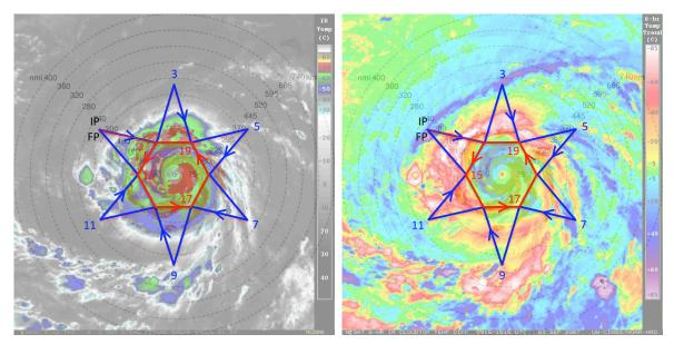
Fig. 4. Same as in Fig. 3, except that a circumnavigation of the storm is performed after (or before) the star pattern is completed. The hexagon circumnavigation that is shown has points that are 90 nm (165 km) from the storm center, but can be adjusted outward for safety considerations depending on the strength and size of the TC.
