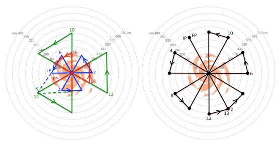
Figure 5. Sample flight patterns for the NOAA SHOUT Global Hawk aircraft. (Left) Series of 3 alternating radial leg butterfly patterns and (right) rotated butterfly pattern with 30 degree rotated radial legs.
