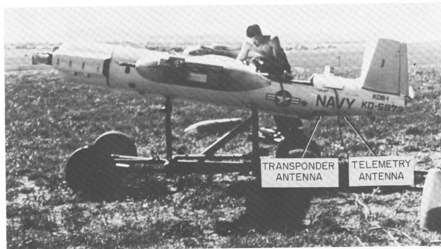
Fig. 1 - Standard target drone modified to expose meteorological sensors on wing pods. Telemetry and radar transponder antennas are visible near the rear of the fuselage.
